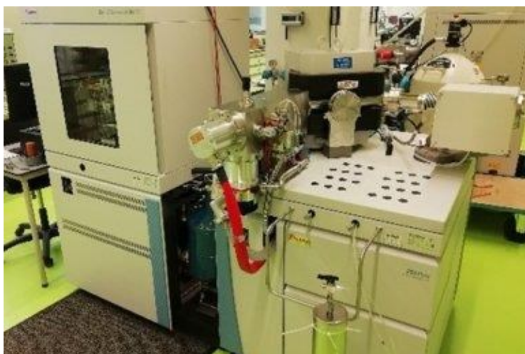
Fig.2.3. Kiel IV carbonate device (left) coupled to a 253 Plus IRMS in the Stable Isotope lab (right), Utrecht University.
