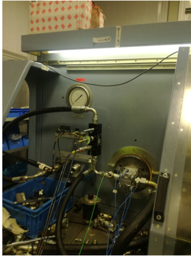
Figure 28: Frontal view of the test bench where the gear pump has been tested
