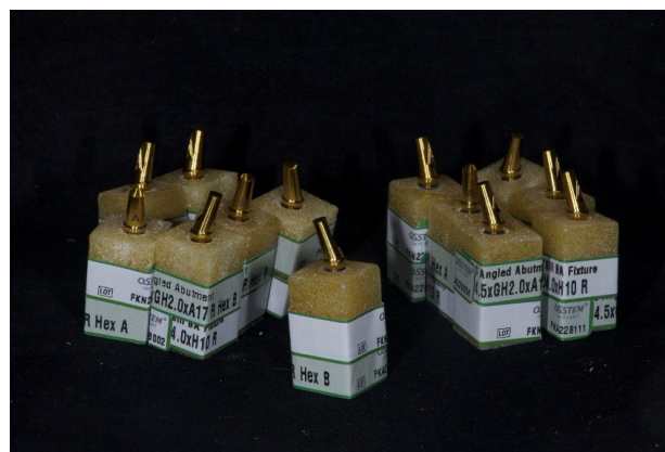
Figure 2. All 13 blocks ready for the static and dynamic loading.
