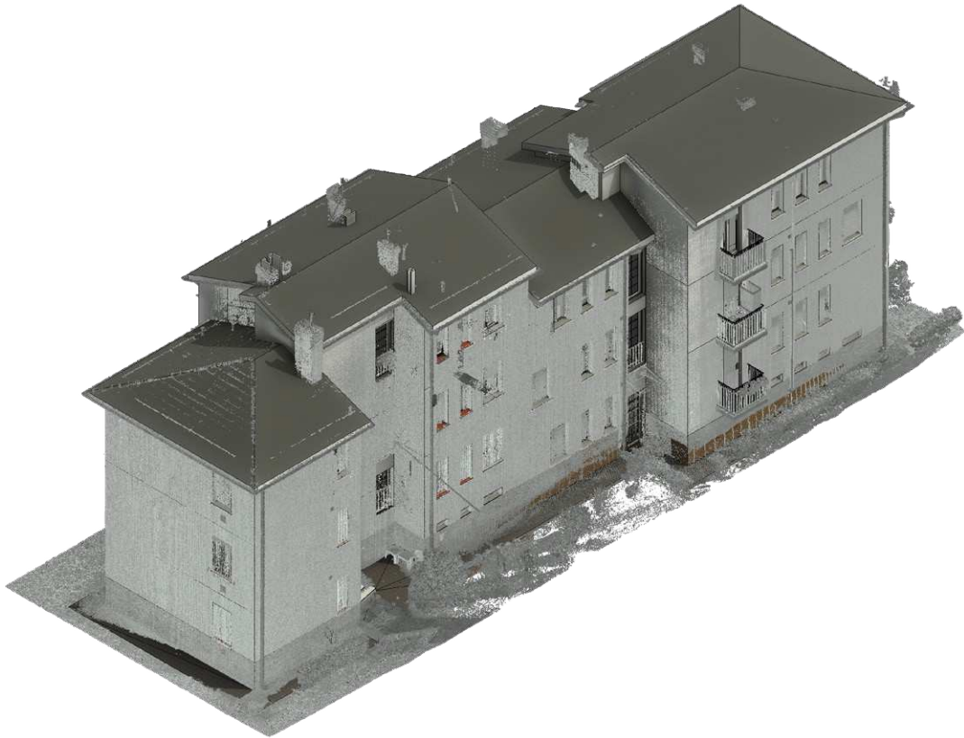
Fig. 020 - Overlaying the model on the point cloud for the deviance verification phase.
