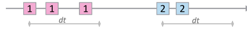
(b) Time proximity between hits. Only hits close in time can be part of the same cluster.
