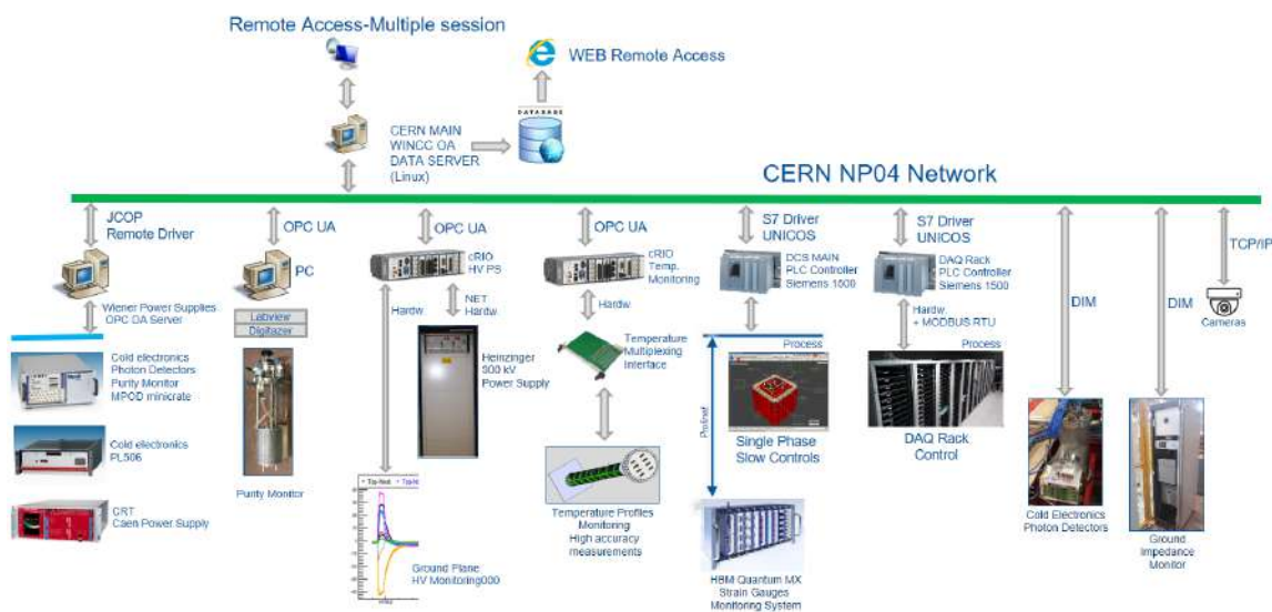
Figure 86. DCS architecture and communication protocols.
