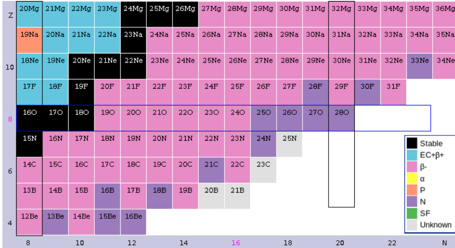
Figure 1.3.: Nuclear chart focused on the neutron-rich region of sd nuclei. The color scheme of the chart represents the main decay mode and the legend is reported on the bottom right of the figure. In particular, the nuclei reported purple decay through neutron emission and are unbound. Figure adapted from [12].
