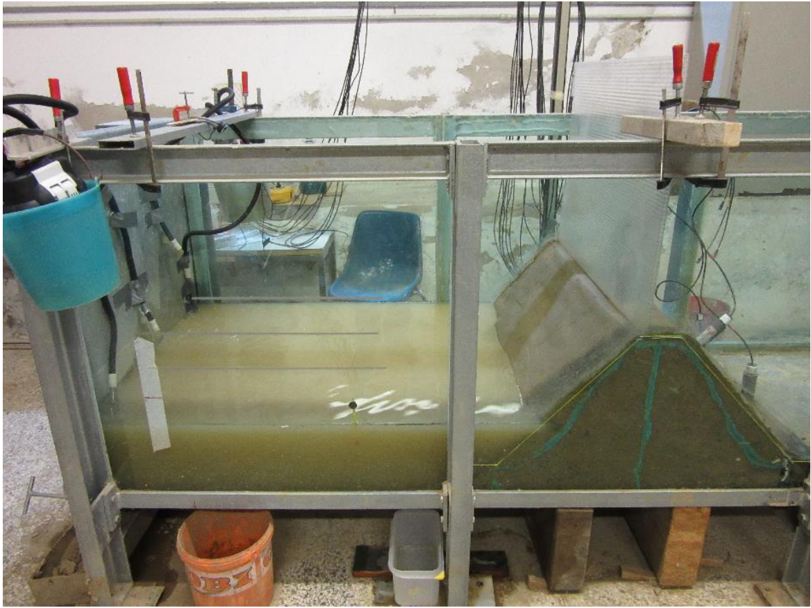
Figure 3: Constructed model levee at DICEA (Department of Civil and Environmental Engineering, University of Florence) 48 hours after release of crayfish into the setup.
