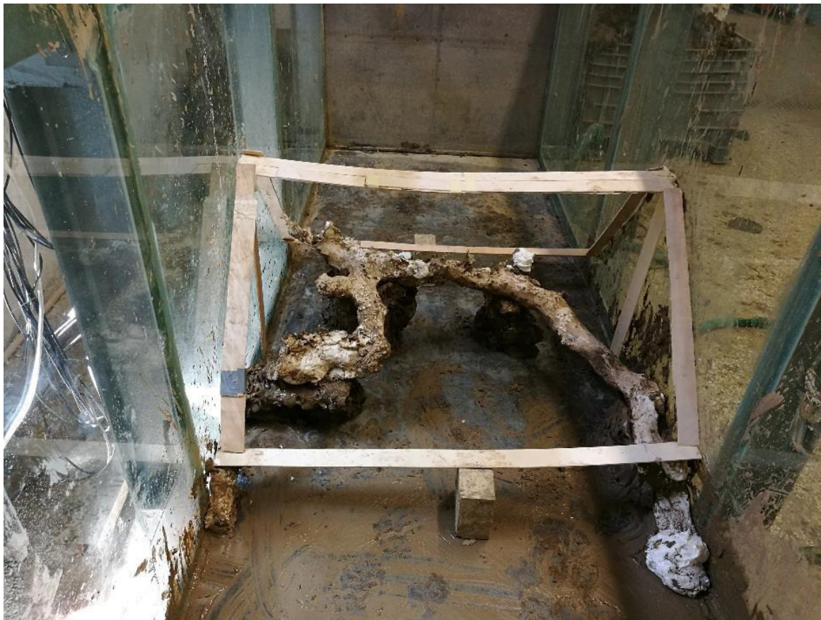
Figure 4: Reconstructed model of the levee after the experiment, showing the position and the excavated volume of burrows.
