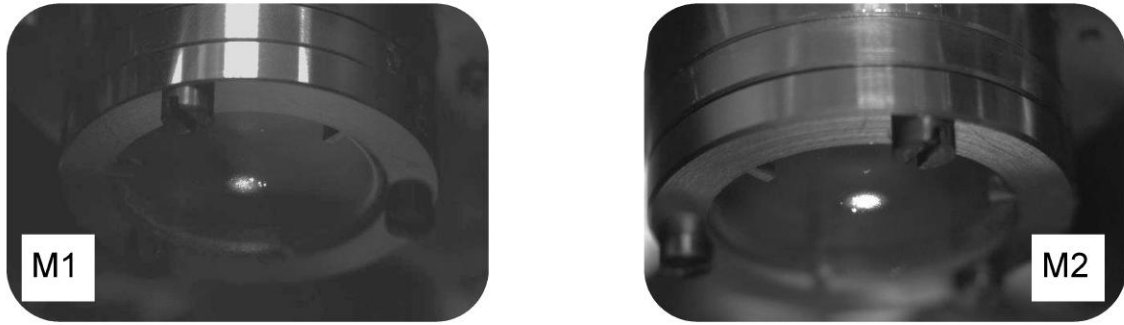
Figure 4.32: Infrared photographs of the reflecting surface of the mirrors with the laser locked to the cavity.
