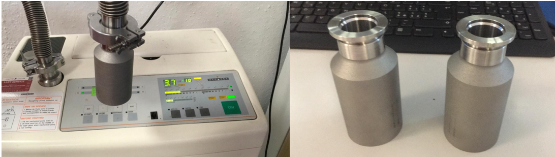
Figure 4.47: Vacuum test of a classical cylinder made in steel-base metal powders material by 3D print.
