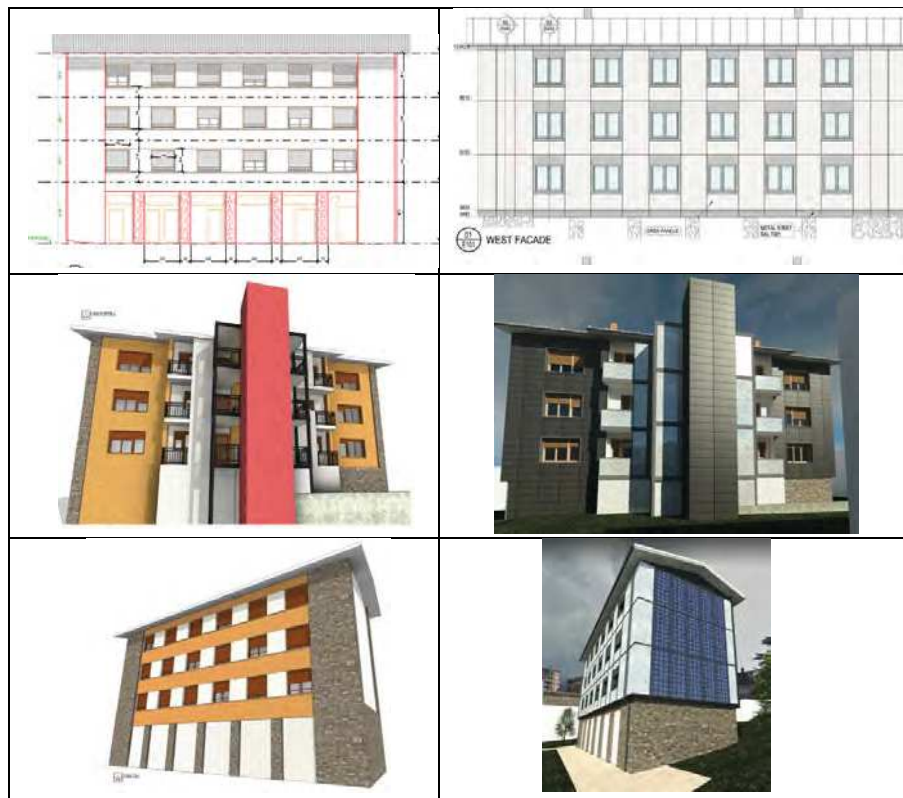
Figure 7: Left: Current stage building drawings in REVIT based on building’s 3D scanning. Right: retrofitting proposal, modules lay out
