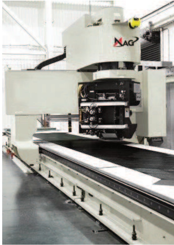
Fig. 1.4: ATL Machine (Photo courtesy of MAG)
