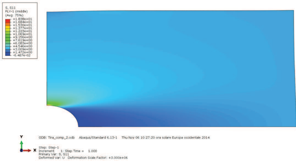
Fig. 5.27: \sigma_x stress of the Ply-1 in x direction
