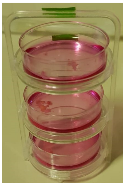
Figure 8.2: Tripod used to host three petri dishes each test, to increase the exhalation surface of the samples.
