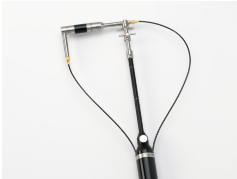
Figure 3.1: Example of Axial p-p Intensity Probe: Microphones are in Face to Face Configuration
