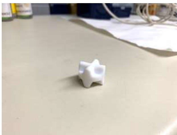
Figure 32: “double-sided crosshead” magnet associated with the magnetic stirrer.
