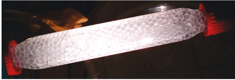
Figure 3.6: Picture of the lab scale photodegradation apparatus with colloidal \text{WO}_3 spheres in static conditions
