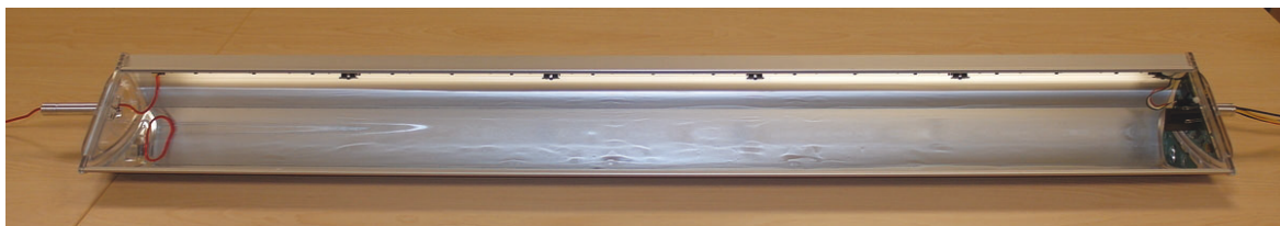
Figure 3.1: Picture of a Solar F-Light ® concentrator for electrical energy production.
