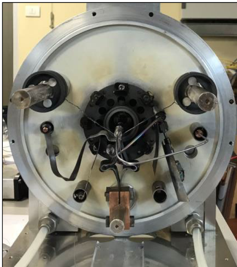
Figure 5.9: The SPES PIS with the oven loaded with Sc(NO 3 ) 3
