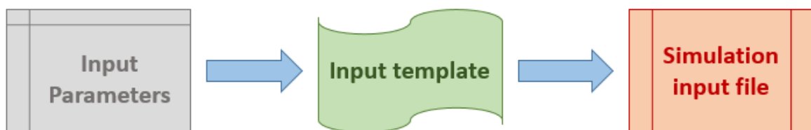
Figure 7.13: A script insert automatically the input parameter in the template for both codes.
