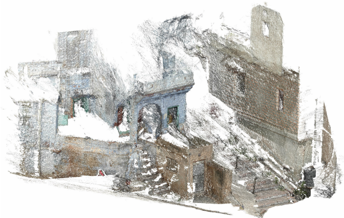
Image 32: Point Cloud created with 16 photos reconstruction thanks to photogrammetry processes of the old centre of Jodhpur, inside one of the case study areas
