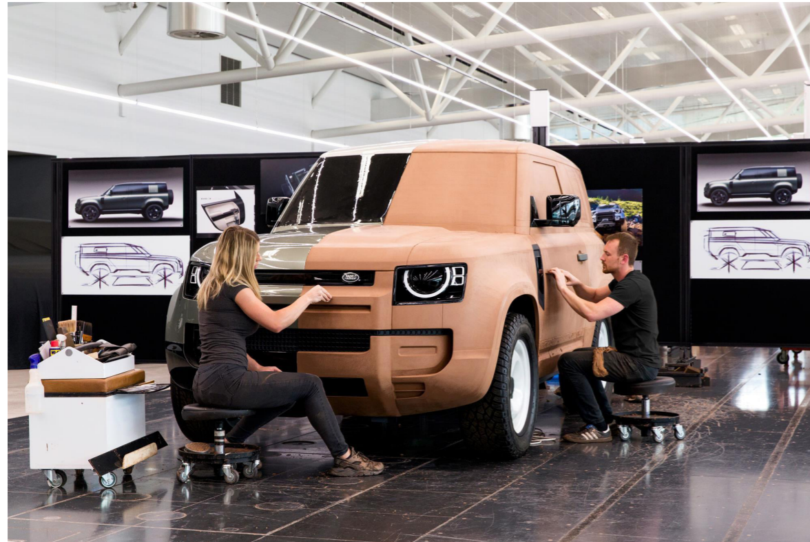
Img. 08 • Stylists are designing a full-scale physical mock-up to represent visually the proposed vehicle during the concept-generation process. The model is very useful to acquire a better feel of the size, space, and configuration of the expected product. Source: Land Rover.
