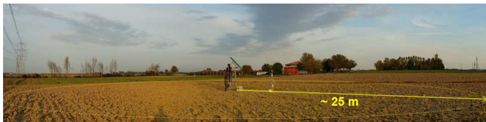
Figure 8.3: representation of the field of vision of NaI(Tl) installed in the Gamma Station at 2.3 m height. In yellow is highlighted the region that produces the greatest contribution in the gamma signal. The percentage of source radiation detected reaches 95% at \sim 25 m (see Section 9.1)
