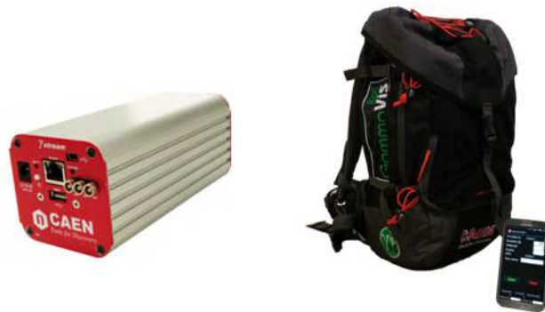
Figure 4.8: the digital multi-channel analyzer GammaStream (left) and The ZaNaI detector (right)
