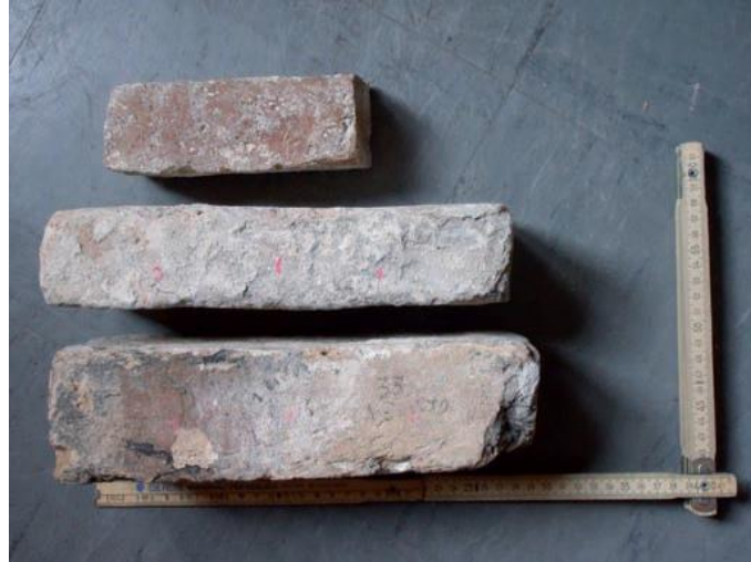
Figure 4.4: different brick formats present in the Po valley (image from Squassina (2011)).
