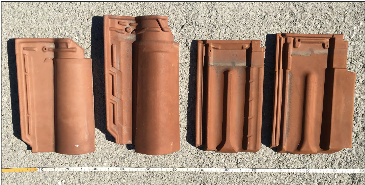
Figure 2 Roof tiles used. From left to right, standard Portoghese, herotile Portoghese, standard Marsigliese, herotile Marsigliese.
