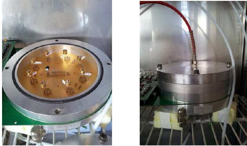
Figure 3.8: Sensor inside the chamber (left) and chamber hermetically sealed (right).
