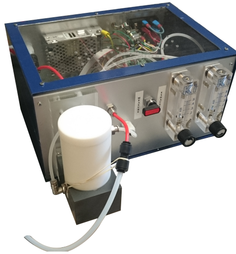
Figure 4.34: The prototype SCENT A2, located at the Sensor Laboratory of UNIFE.
