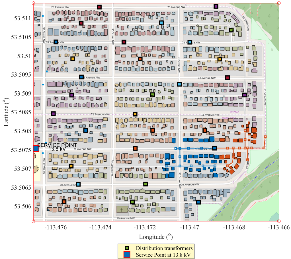
Figure 4.9: Case study 1: Low voltage distribution network, where distribution transformers and end users are represented with different colors depending on the cluster.
