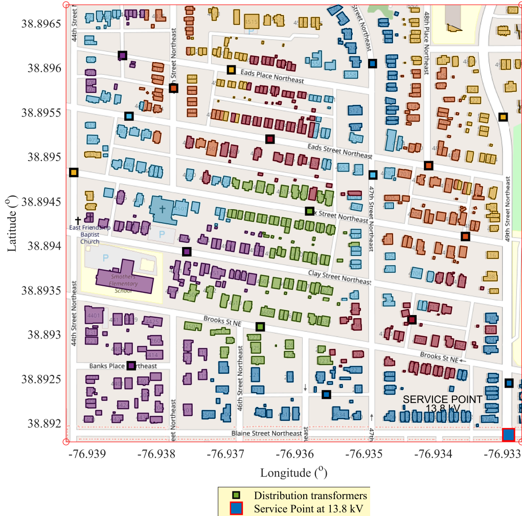
Figure 4.10: Case study 2: Low voltage distribution networks, where distribution transformers and end users are represented with different colors depending on the cluster.
