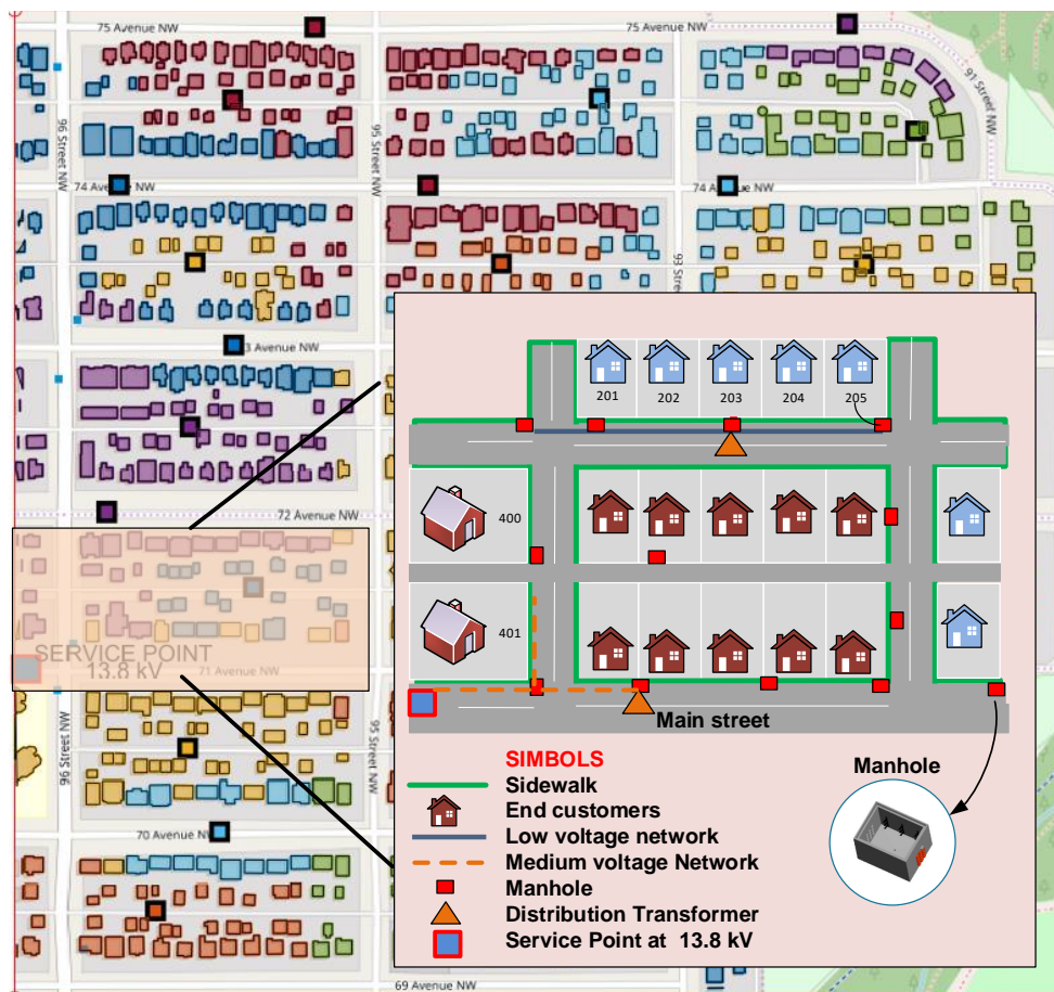
Figure 4.7: A schematic overview of the distribution network and its main components.
