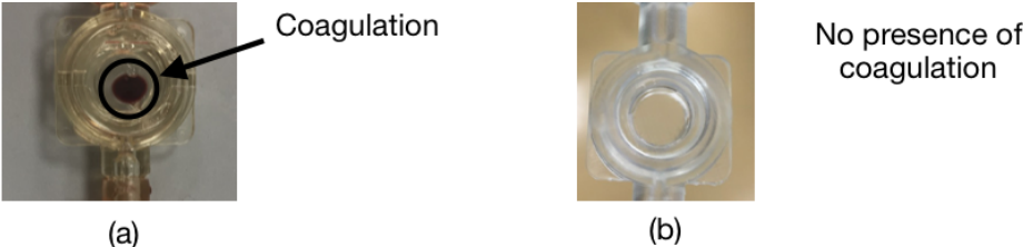
Figure 1: Two cuvettes after a session of dialysis. (a) shows the presence of a coagulation, while (b) does not show the presence of coagulation
