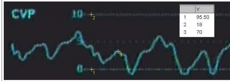
Figure 2.5: Calibration of the y scale: 1 and 2 are the inferior and superior points on y axis, 3 is one point Y on the trace.
