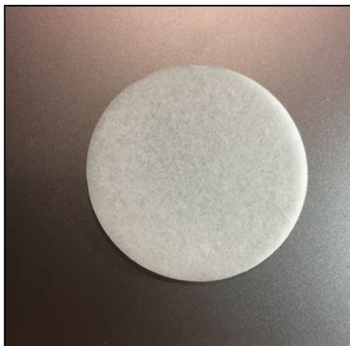
Figure 3.16: NaNO 3 disk with 40 mm diameter, usable as secondary target for the Ag deposition tests.
