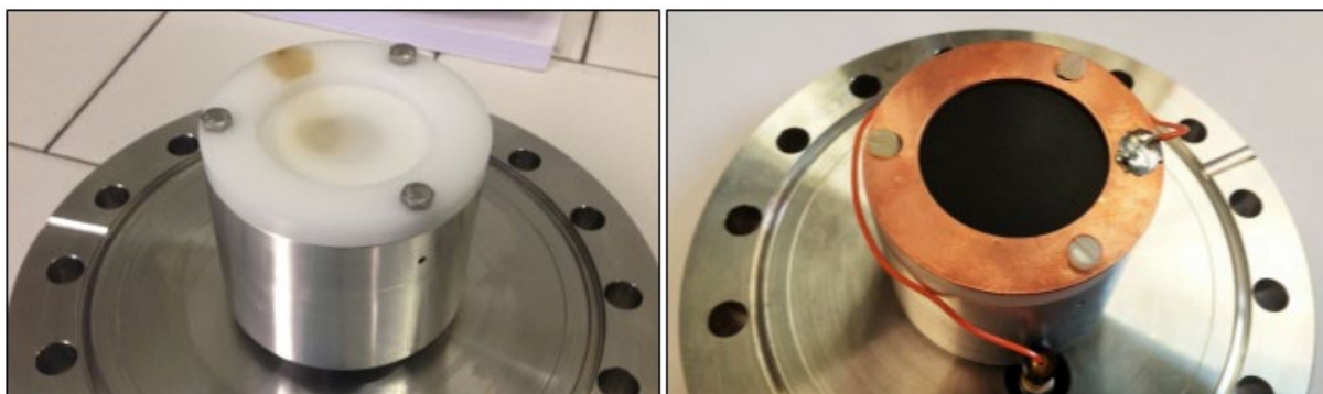
Figure 3.13: the collection targets used for the Sr, Y and I deposition tests, that were assembled directly to the closing flange of the FE beam line. On the left the NaCl disk used for the Sr and Y tests, whereas on the right the activated carbon disk used for I.
