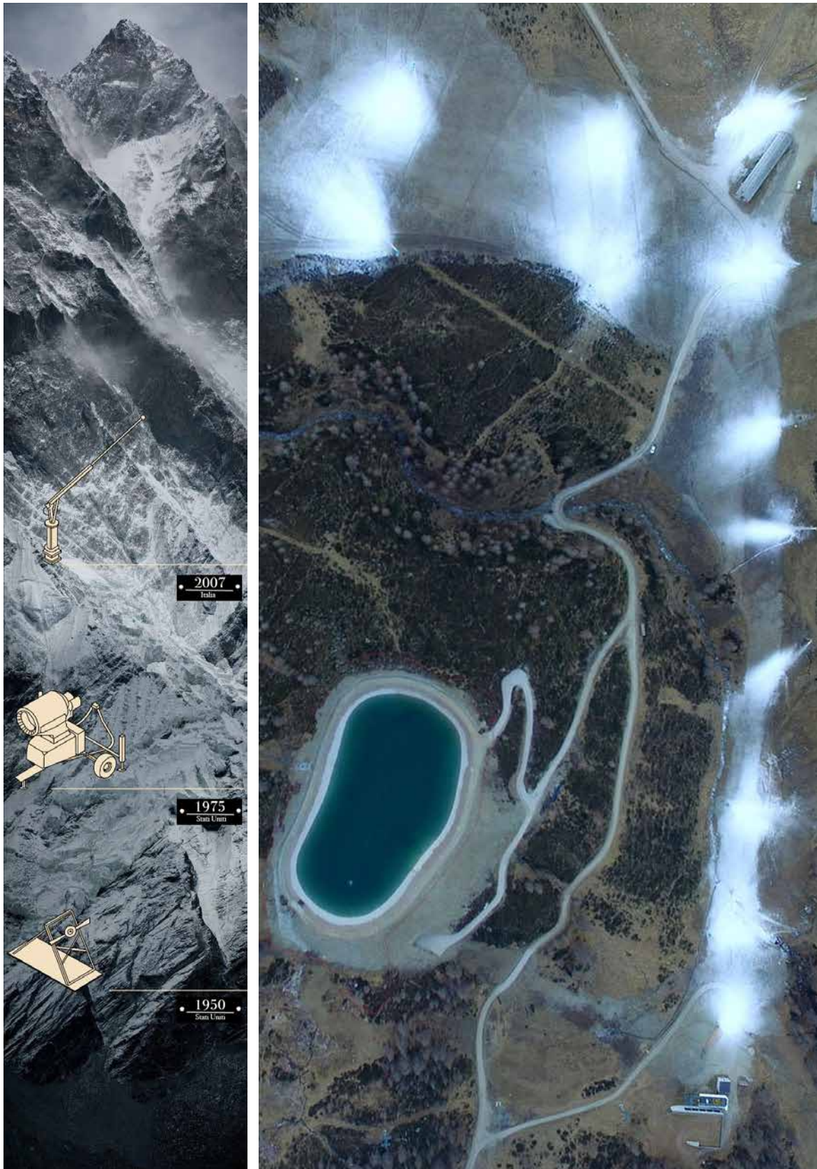
Figure 4.7: The image shows snowmaking operations and some of the infrastructures used to make it possible such as water basins, pumping stations, tanks, cannons, electricity networks, etc.
