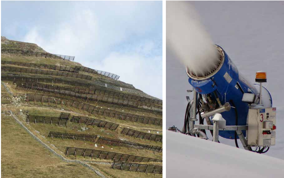
Figure 4.8: Two of the main operative tools used to manage the touristic landscape of ski resorts: avalanche protection barriers and snowmaking cannons.
