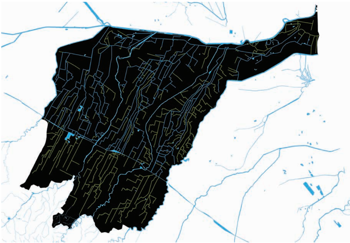
Figure 3.32: The two figures show the Consortium lowland district; above, the water drainage system composed by drainage (in green) and mixed-use canals (in blue); below, the irrigation system composed by pressured pipes (in red) and mixed-use canals (in blue).
