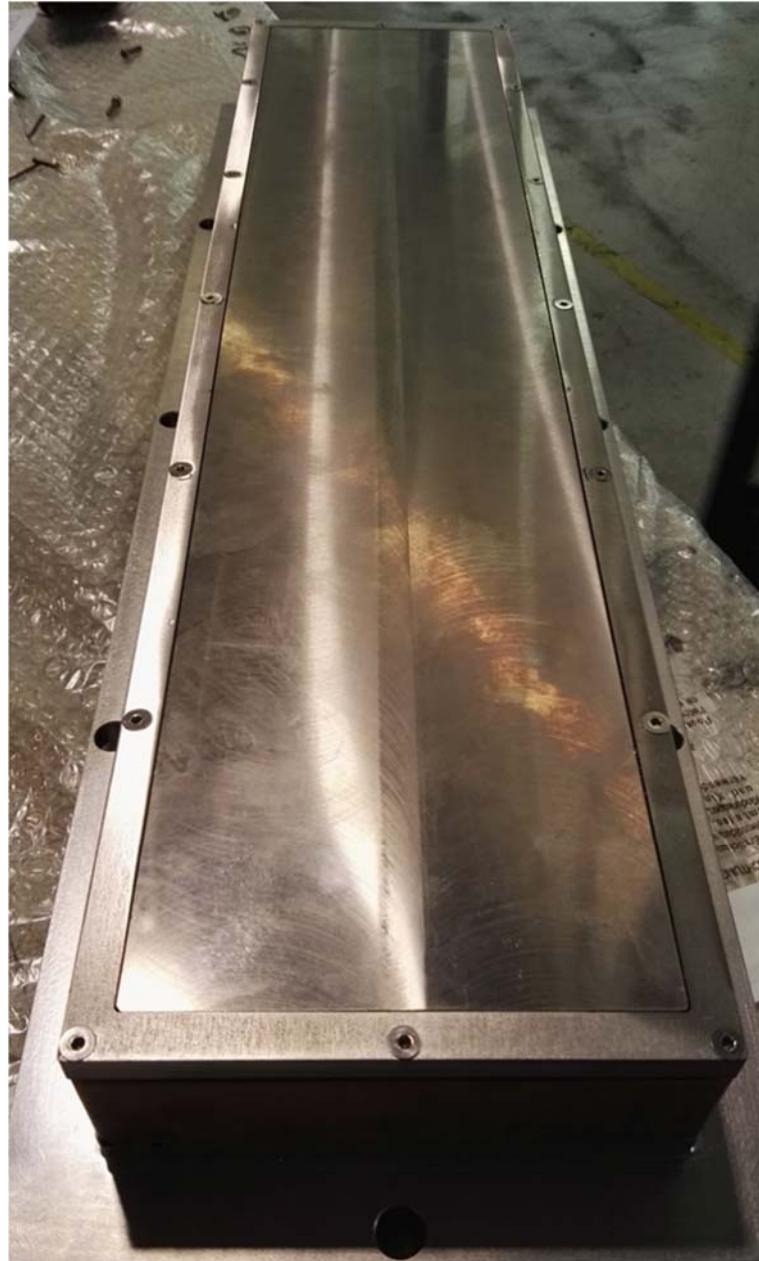
Figure 64: magnetron sputtering source ready for the assembling onto the industrial PVD system.
