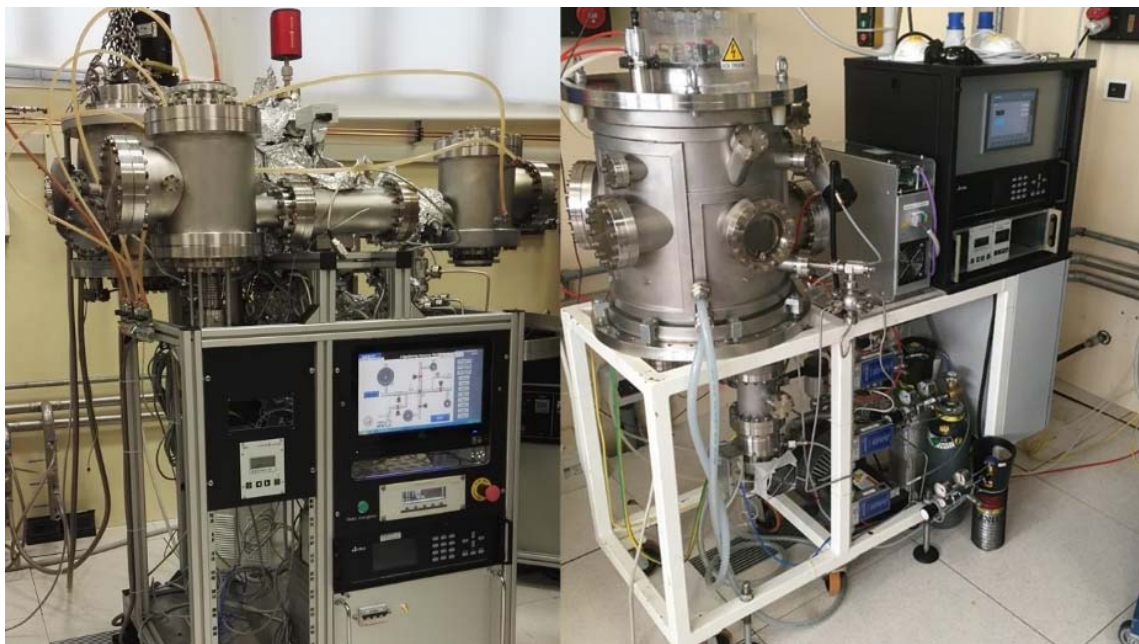
Figure 21: the PVD system prototypes located in the Material Science and Technology for Nuclear Physics Service at the National Laboratories of Legnaro. On the left the four chambers system dedicated to the magnetron sputtering and on the right the prototype dedicated to the cathodic arc deposition.
