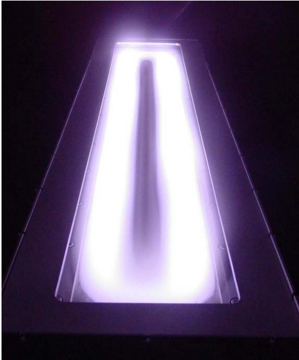
Figure 8: plasma of a magnetron sputtering rectangular source 12 .
