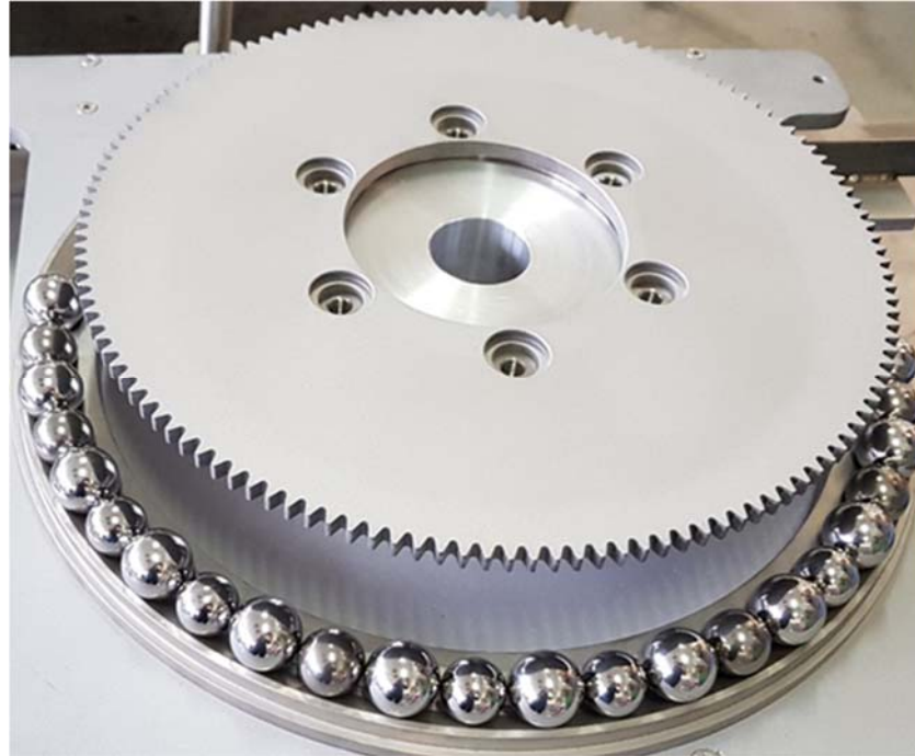
Figure 74: the base of the sample holder evidencing the spheres used to dissipate the weight and maintain the rotation.
