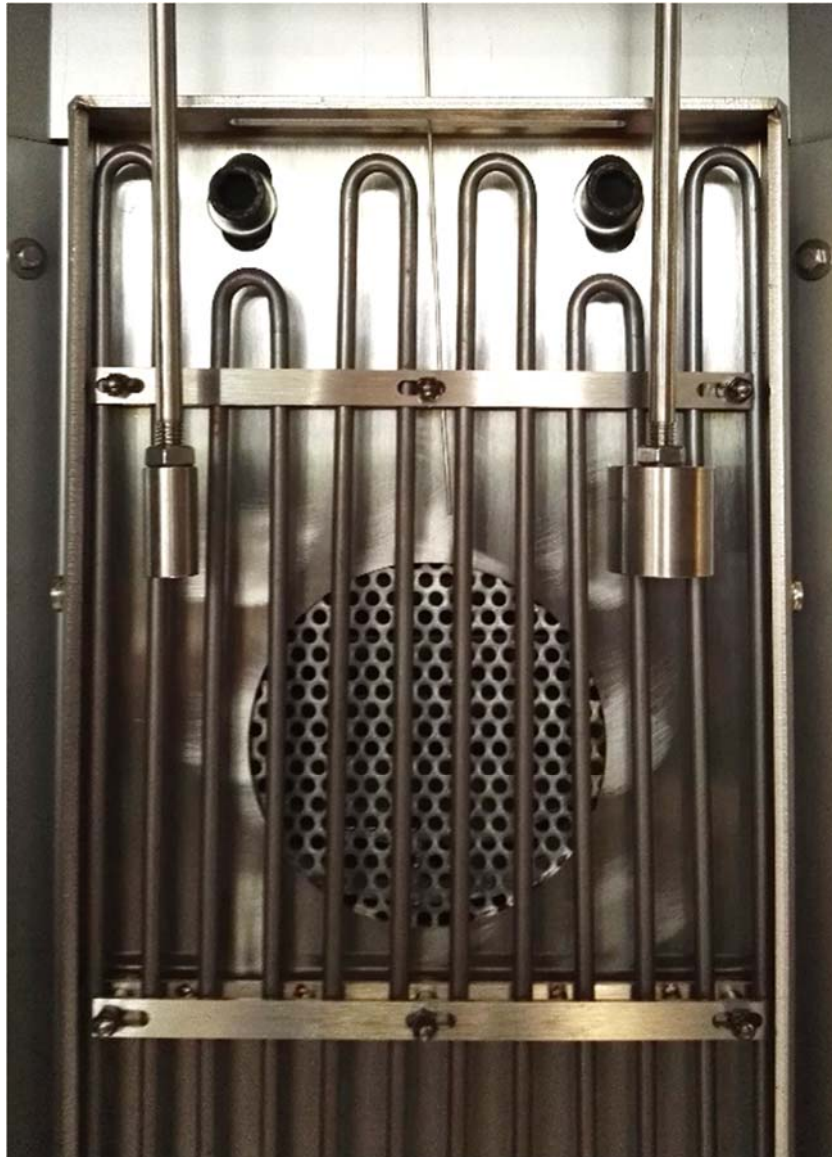
Figure 68: detailed view of the resistive heater positioned in correspondence of the pumping flange.
