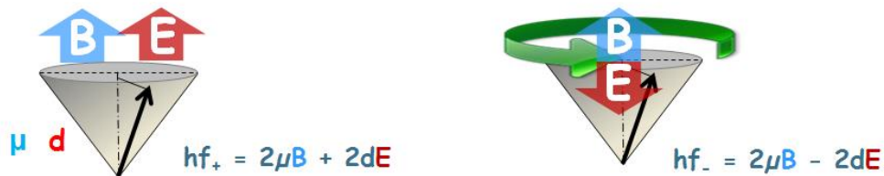
Figure 1.2 - 'Traditional' approach for EDM measurement, limited to neutral particles, atoms or molecules. \mu = Magnetic Dipole Moment, d = Electric Dipole Moment, B = Magnetic field, E = electric field, hf = spin precession frequency.
