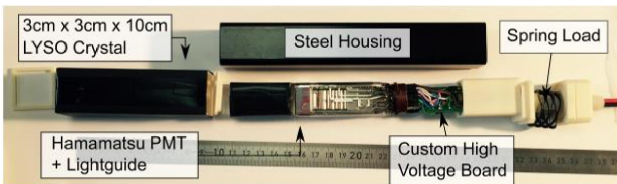
Figure 4.7 - Detailed view of a single LYSO module, coupled with an Hamamatsu PMT, as used in LYSO I experiment
