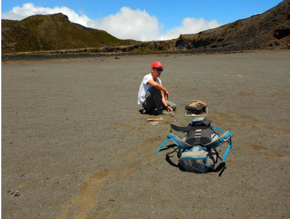
Figure 8. Sampling soil CO 2 gas by the dynamic method in the Karthala summit area
