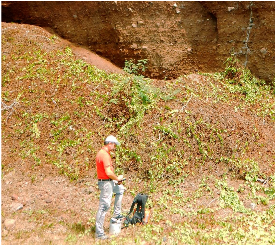
Figure 9. Sampling soil CO 2 gas by the accumulation chamber method at Petite Terre
