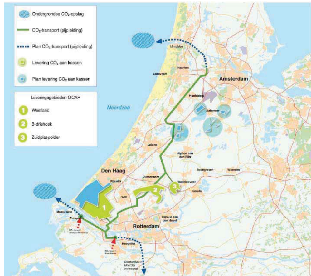
Fig. 172 OCAP pipeline (source: Ros, M. et al., 2014)
