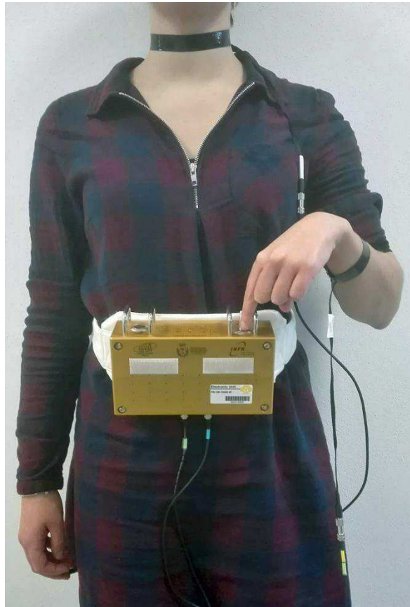
Figure 4.4: Plethysmography system fixed at the waist of the subject. Arm and neck sensors are connected to the PEU.
