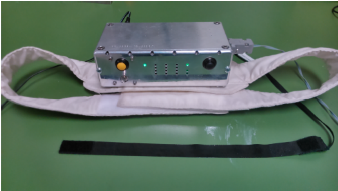
Figure 4.3: Portable electronic unit (PEU). This unit allows the connection of three different capacitive sensors, Li-ion battery or external power supply, SD card for data storage and serial cable for the transmission of the acquired data.
