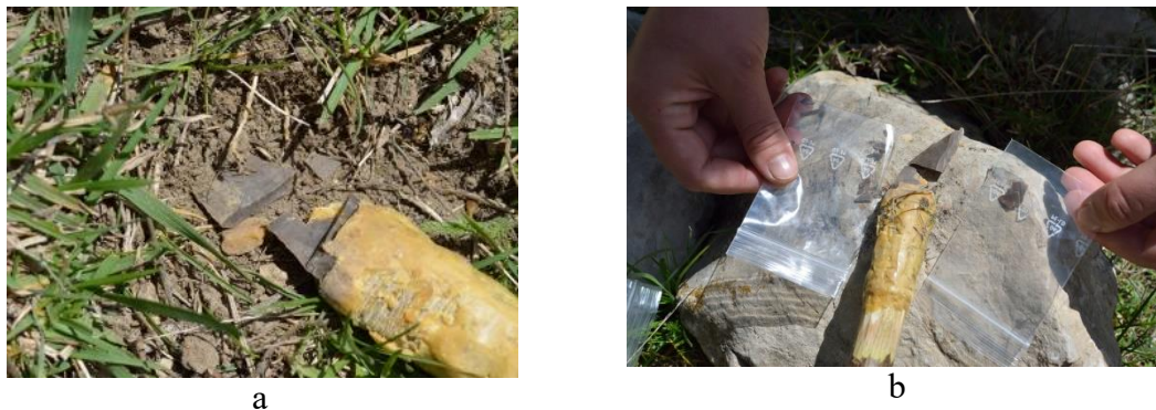
Figure 4.6: Zaragoza no 2 (spearhead, 1 shot was performed) (a) showing the spear point embedded inside the sediment till the hafting area (b) micro-chips happened due to impact fracture
