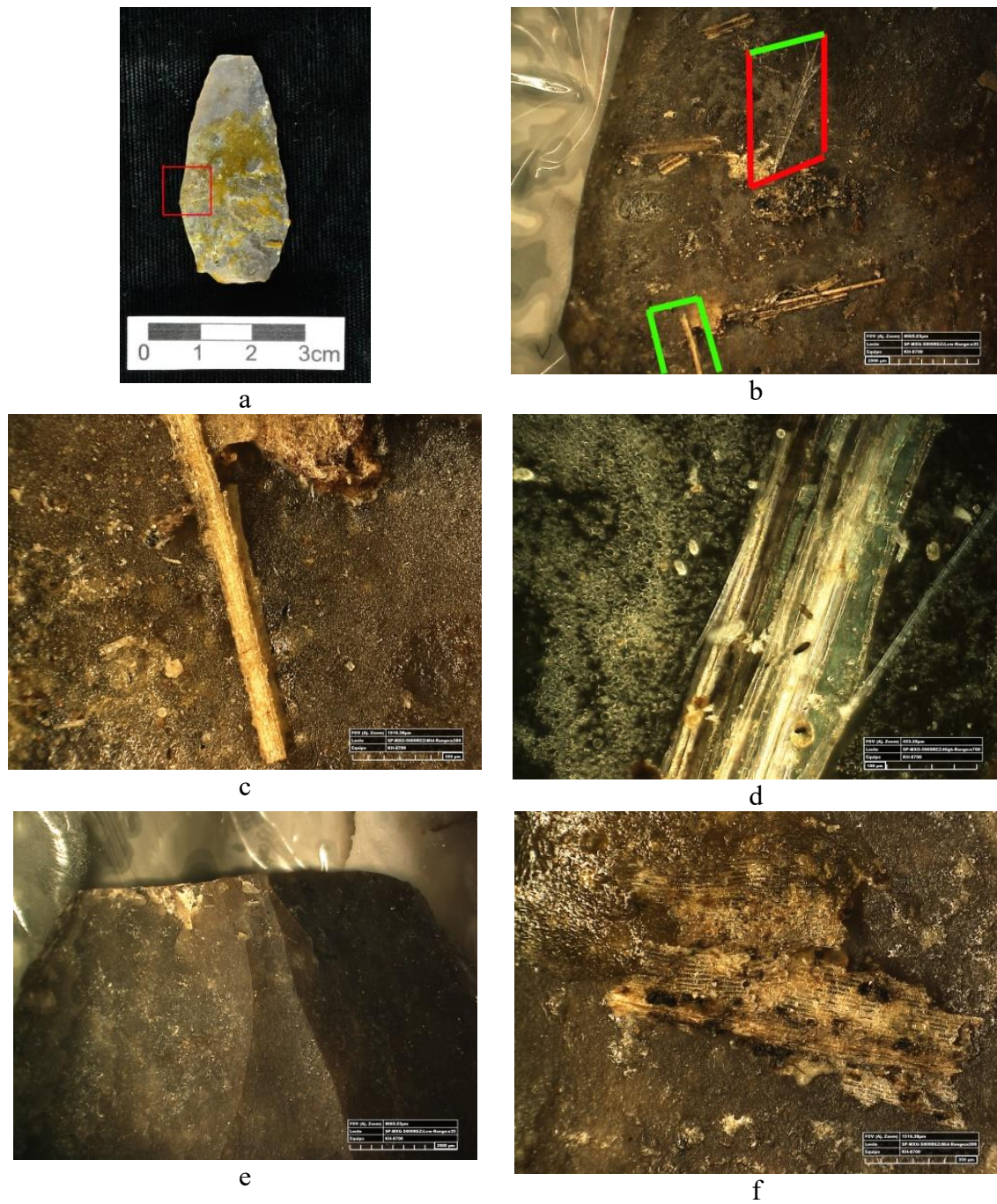
Figure 4.10: Zaragoza no. 3 (arrowhead, 1 shot was performed) (a-b) showing the locations of residue; (c) plant residue at 140x; (d) plant residue at 700x; (e) tip fracture on dorsal side at 35x; (f) adhesive residue with the industrial twine impression on it at 200x
