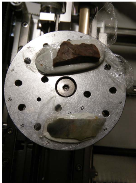
Figure 3.3. In the SEM chamber, archaeological tools placed on the molding clay which is covered with cling plastic film
