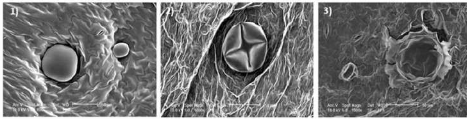
Figure 5. Effect of power ultrasound on boldo leaves: 1) control leaf surface, 2) leaf surface after conventional process, 3) leaf surface after UAE (Chemat et al., 2017).
