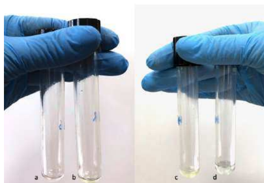
Figure 53. SFE extracts (a: SFE wheat aleurone; b: SFE rice bran; c: yellow corn SFE; d: white corn SFE) (photo credit: Ilaria Burlini)
