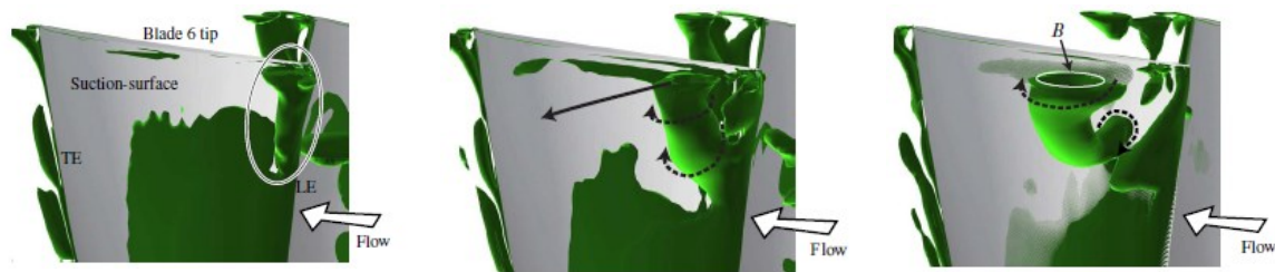
Fig. 2.38 - Formation of the Tramped Shaped Vortex: (a) leading edge separation circle; (b) vortex tube forms, uppers and moves circumferentially along casing; (c) lower end of tube moves downstream along suction surface; (taken from (Pullan, et al., 2015))
