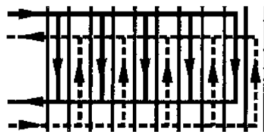
Figure 9: counterflow, 1 pass - 1 pass plate HE scheme (from [23])
