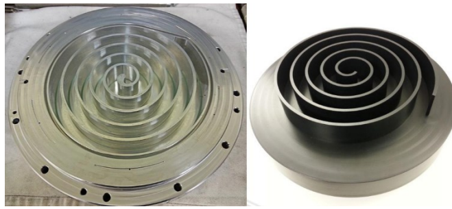
Figure 13: disassembled scroll machine; stator (left), rotor (right)
