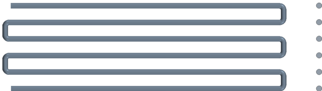
Figure 60: geometry of the heat exchanger. A transversal section is showed on the right
