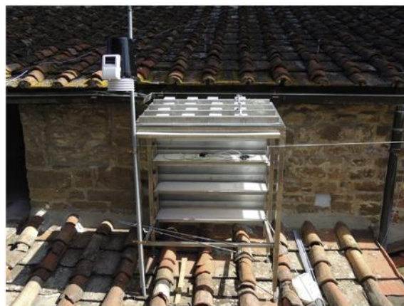
Fig. 1. Carrara marble model samples exposed on the rack at Santa Croce Basilica, Florence.
