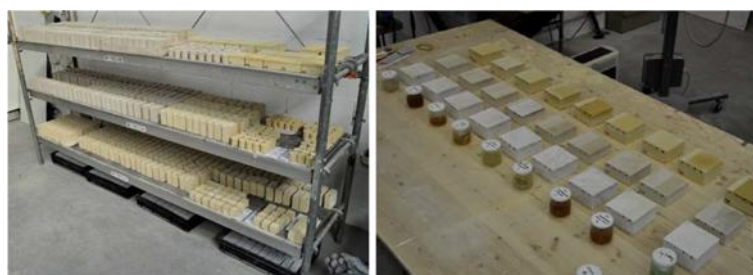
Figure 2 Samples of the stones selected for testing (left); application trials on different lithotypes (right).
