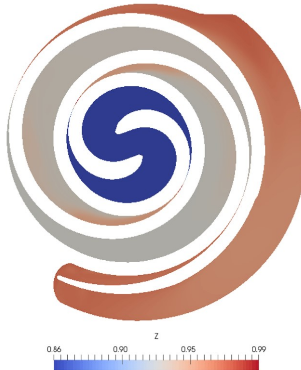
Figure 5.13: Compressibility factor for R134a during the operation of the expander [59]
