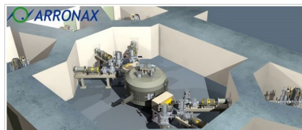
Figure 9 Graphical representation of the IBA cyclotron installed in ARRONAX facility.
