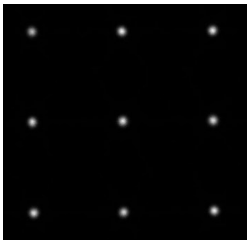
Figure 21 Planar image of the grid phantom obtained using cyclotron-produced ^{99m}\text{Tc}[\text{TcO}_4^-] 8 hours after EOB.
