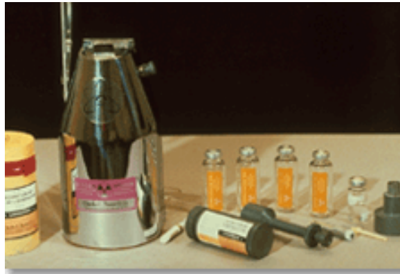
Figure 2 Picture of a commercial {}^{99}\text{Mo}/{}^{99\text{m}}\text{Tc} generator.
