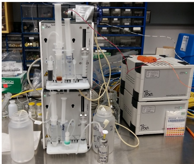
Figure 34 Picture of the assembled IBA module for the extraction and purification of Tc-99m from the molybdenum metal target.
