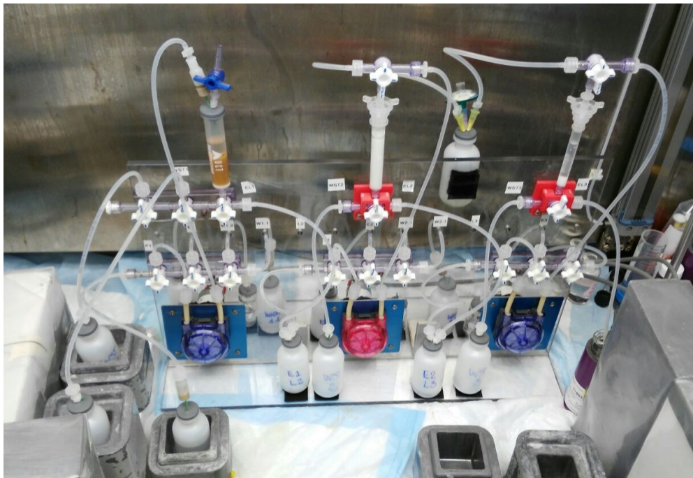
Figure 59 Three pumps semi-automatic module.
