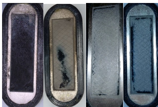
Figure 29 Targets after molybdenum dissolution tests (From left #1 to right #4).
