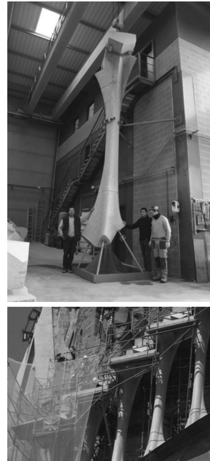
Fig. 4.16 Full scale Passion Façade columns, ready to be installed. Source: ivi, Manufacturing the Bespoke . p.53.
