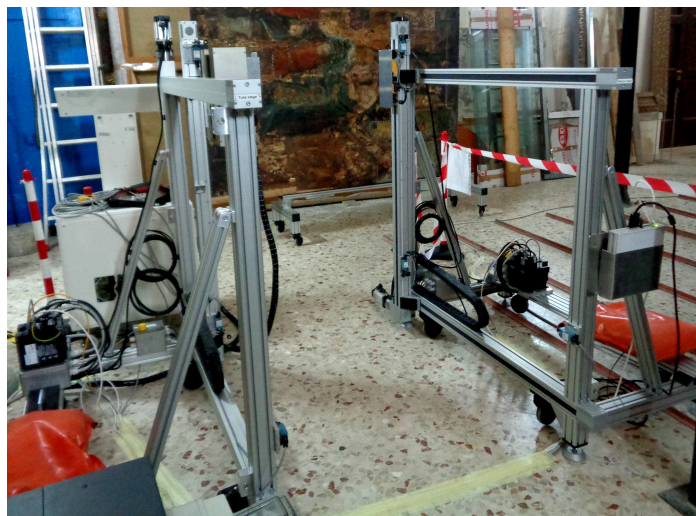
Figure 2.18: The new radiographic scanner at the Regional Gallery of Palazzo Bellomo, Siracuse
