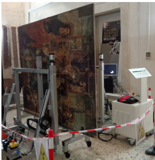
Figure 2.20: Photo of the new RX scanner at Palazzo Bellomo during the acquisition of the RX of the Virgin Mary in throne with the Child
