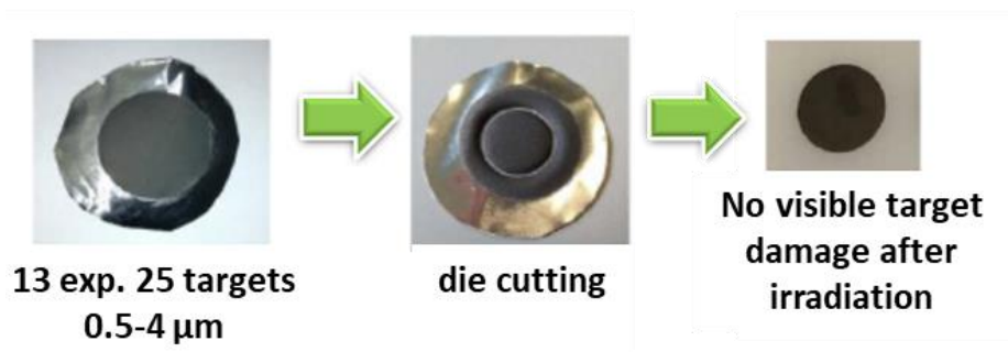
Figure 49: ^{48}\text{Ti} target realized (left), cut with a 12 mm die fitting the target-holder dimensions (middle) and the irradiated target without visible damages (right)
