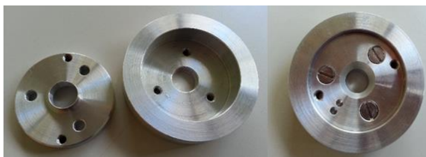
Figure 24: Picture of the dedicated target holder (open and closed)
