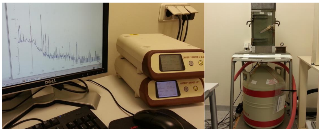
Figure 27: HPGe detector, a digital multichannel analyzer and the computer with the acquisition program, used at ARRONAX to acquire spectra
