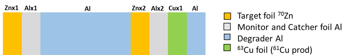
Figure 22: Graphical representation of the staked foil target configuration
