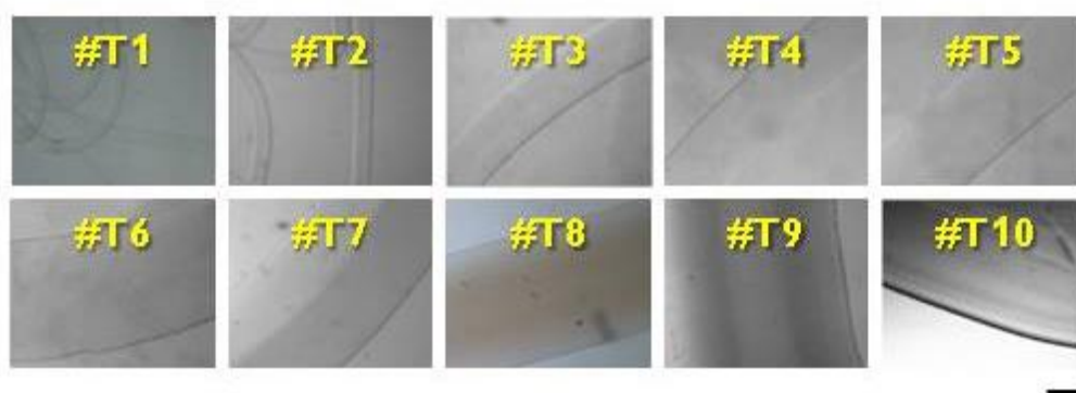
Figure 2.1.3: effect of the microchip outlet tube on the dimensions and morphology of the obtained microfibers. The identification codes, dimensions and material of the outlet tubes are reported in Table 1. Bar corresponds to 500 \mu\text{m} .
