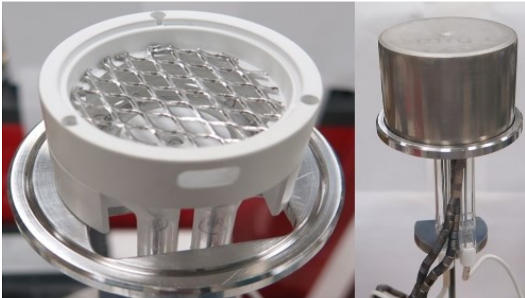
Figure 4.32: D40mm IR lamp driven vacuum brazing furnace.
