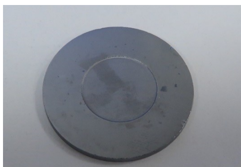
Figure 4.5: Zero-background silicon sample holder for low quantity of powders.
