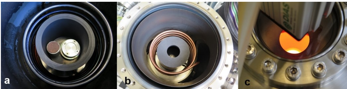
Figure 4.30: Inductive brazing furnace: a) samples positioning, b) graphite chamber closed, c) pyrometer temperature control.
