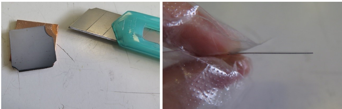
Figure 5.9: 200µm self-sustaining Nb-15 film deposited with program at r.t.
