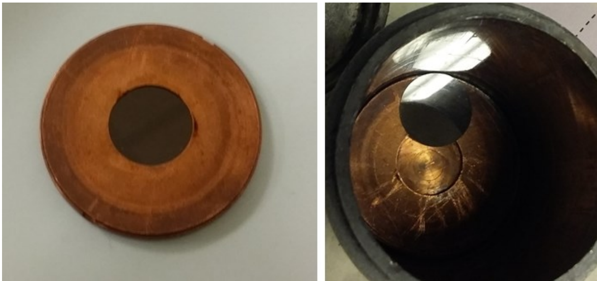
Figure 5.56: CVD synthetic diamond irradiation test in 4-pin clamping target-holder.
