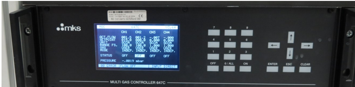
Figure 4.15: MKS multi gas controller 647C.
