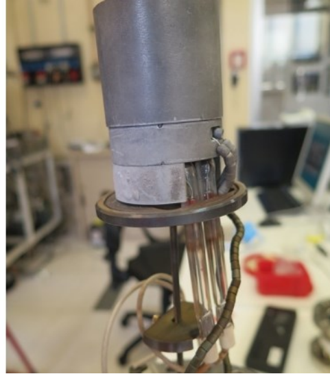
Figure 5.47: Experimental set-up for measurement of relative thermal conductivity
