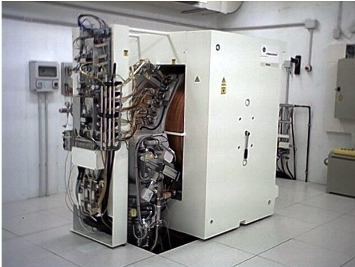
Figure 4.38: GE PETtrace cyclotron of S. Orsola-Malpighi Hospital, Bologna.
