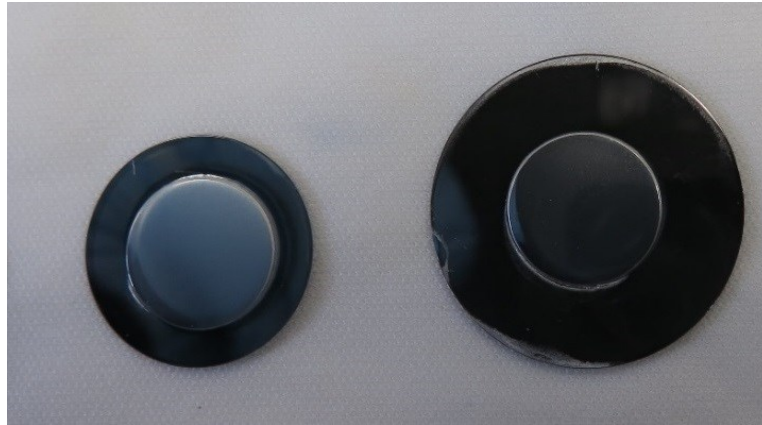
Figure 5.24: Mo-6 and Mo-7 110µm thick Mo sputtered onto sapphire to be brazed to Cu.
