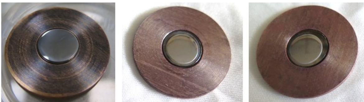
Figure 5.40: S-3, S-4, S-5. Brazed D13 sapphires with Mo film sputtered to copper.
