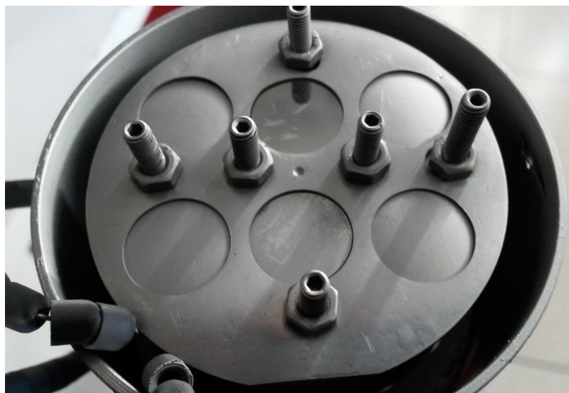
Figure 5.67: Substrate-holder with mask and six D13 substrates sputtered by Mo.
