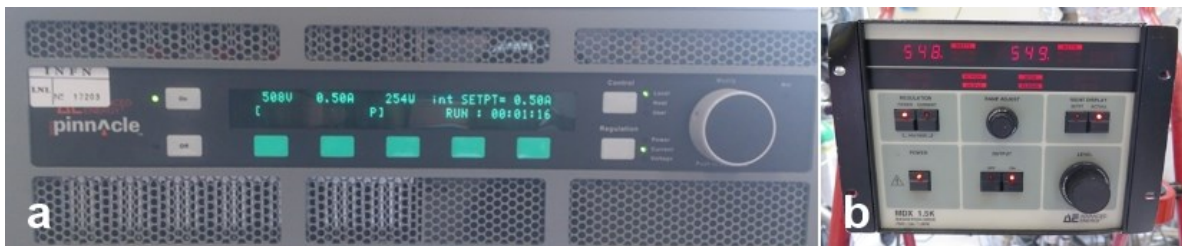
Figure 4.23: DC power-supplies used for magnetron sputtering.
