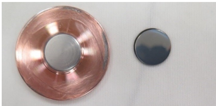
Figure 5.23: Mo-4 and Mo-5 110µm thick Mo sputtered by multilayer approach at 500°C.
