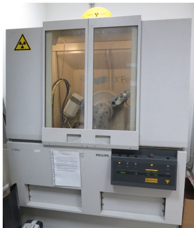
Figure 4.3: X'Pert Philips PW3040/60 diffractometer.
