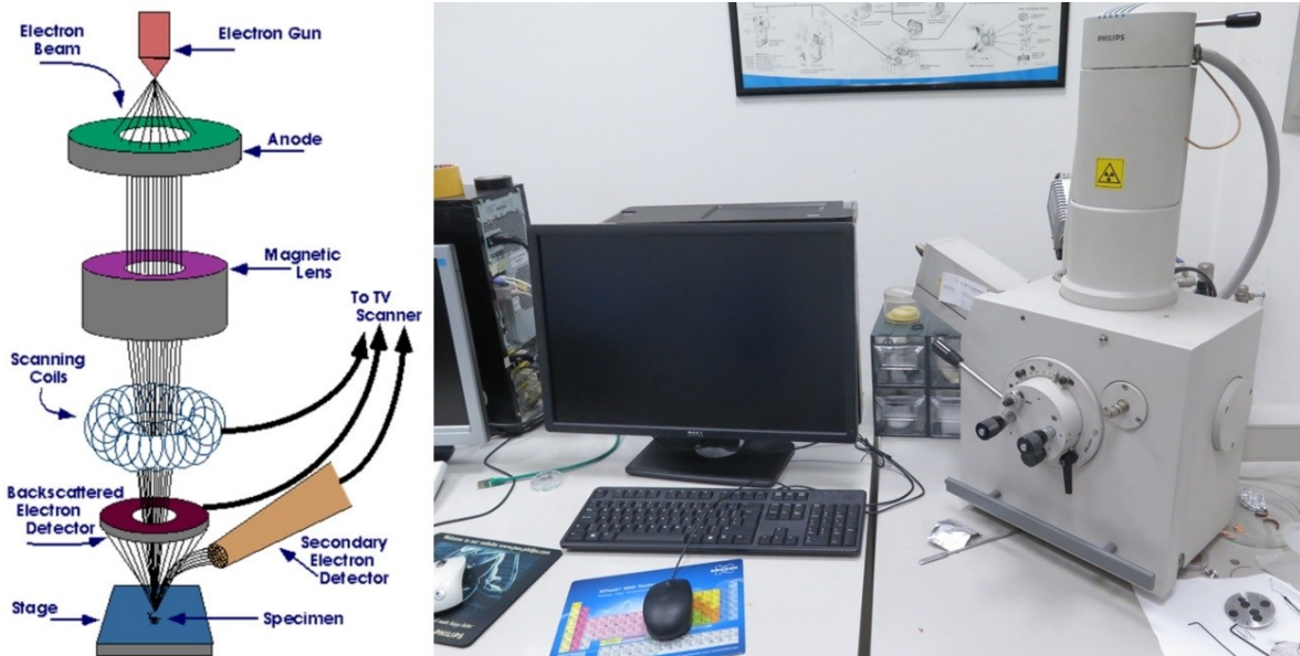
Figure 4.6: a) Basic components of SEM; b) XL-30 Philips SEM with QUANTAX EDS of Bruker
