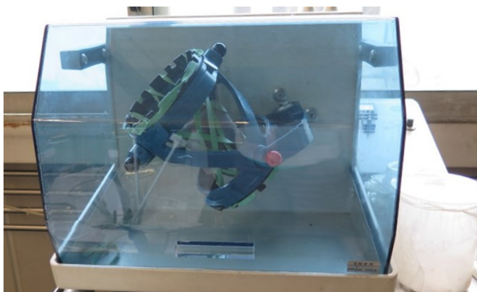
Figure 4.36: TURBULA® shaker mixer for powders.
