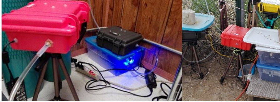
Figure 15. First experiment. Y-PODs boxes for temperature and humidity control experiment. The red case was used outside without any temperature or humidity control for this experiment, instead the black case was used within a shelter where the temperature was controlled to be about 20°C.
