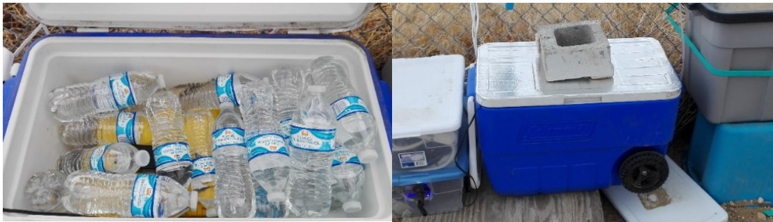
Figure 16. Second experiment. Y-POD box inside the cooler for temperature and humidity control experiment. The previous red case (fig.15) was set up into a cooler with many bottles of a water, trying to have a minimum control on the temperature.
