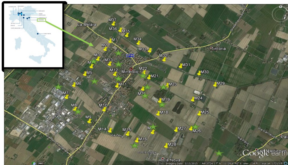
Fig.4 Gas survey measurement, Minerbio area. The yellow color specify all locations under gas monitoring control, the green color specify the Wells used for the Gas Storage activities, all of them surrounding the Minerbio city.
