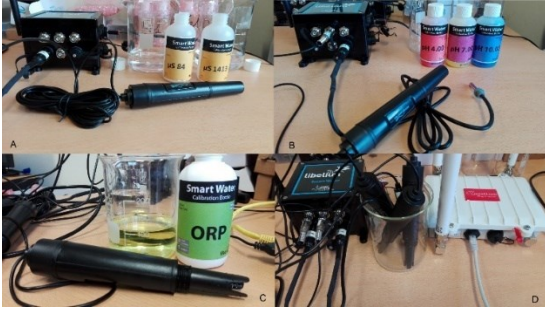
Fig 6: Calibration sensors EC, pH, ORP, and Waspnote node with the Meshlium (Gateway).
