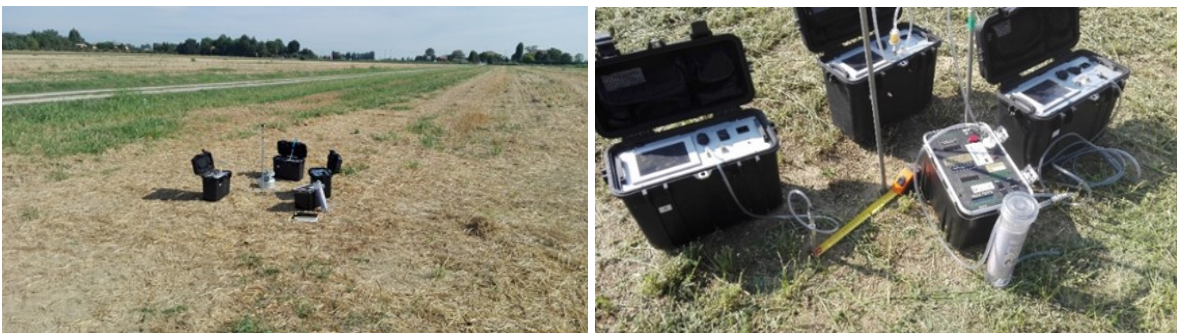
Fig.5 Instruments used during gas survey measurement, for methane and radon concentrations. The three ETG devices were used for methane concentrations and the DurrIDGE RAD7 device with the drierite was used for radon concentrations.
