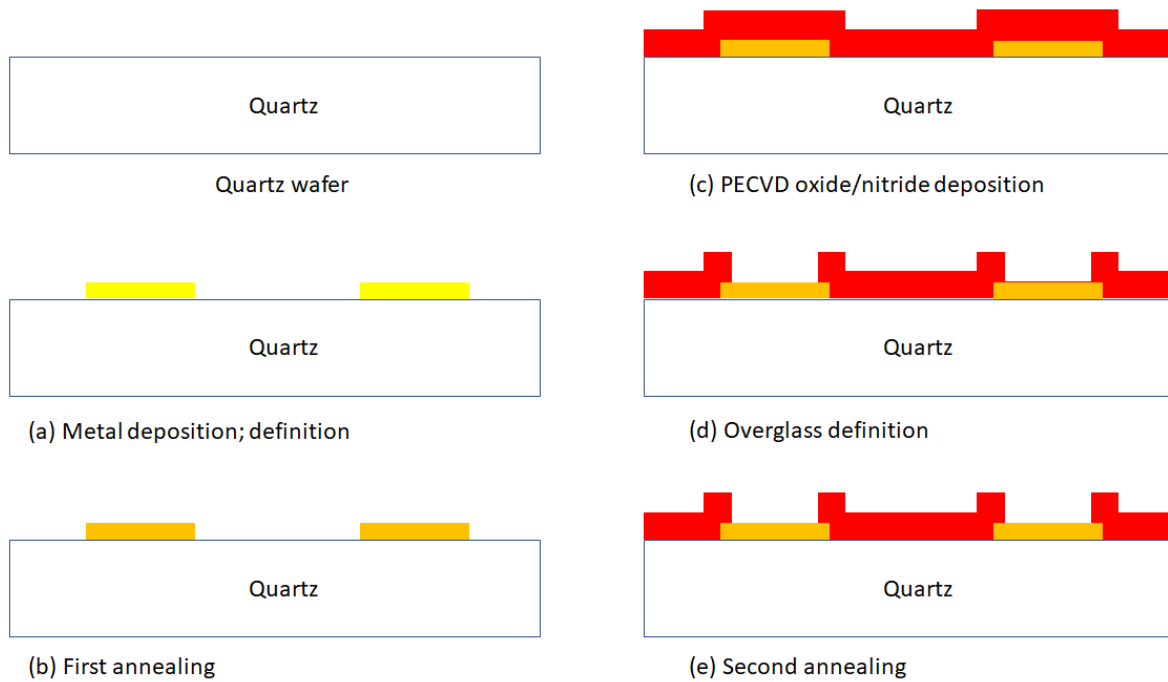
Figure 3.8: The schematic representation of P1Q process steps.
