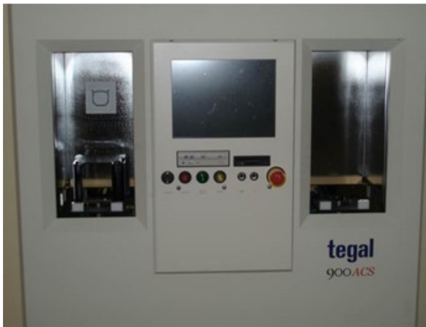
Figure 3.14: The reactive ion etcher OEM Tegal 903 ACS, available in FBK.
