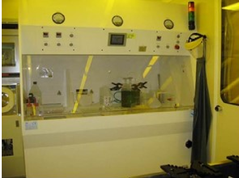
Figure 3.13: One FBK station for wet etching in photolithography processes.
