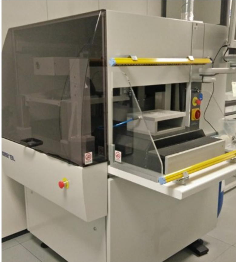
Figure 3.66: Stencil Screen Printer Mod. AUREL Mod. VS1520A used in FBK to deposit sensing material on silicon and quartz substrates.
