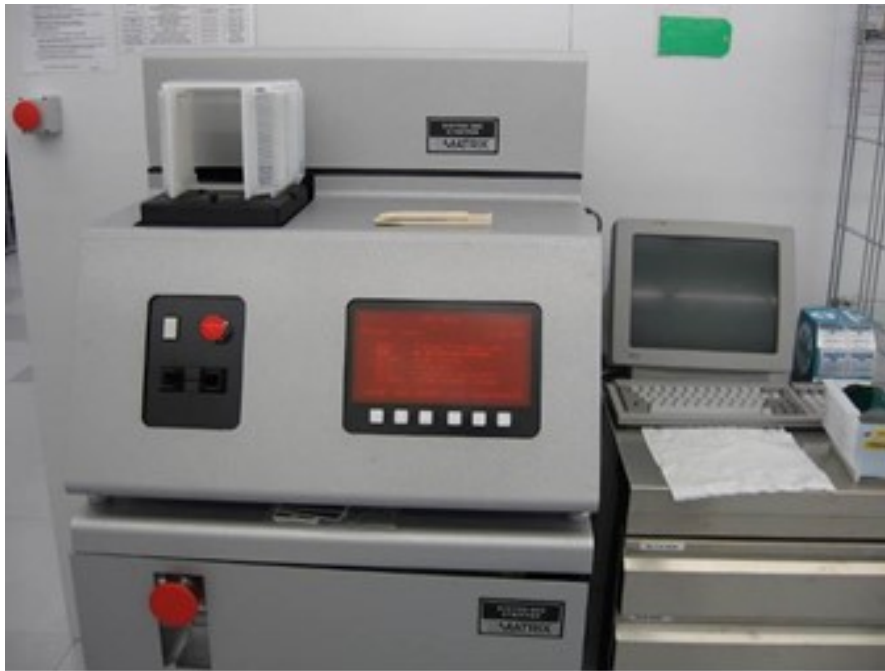
Figure 3.15: The dry stripper Asher, type Matrix System One, available in FBK.
