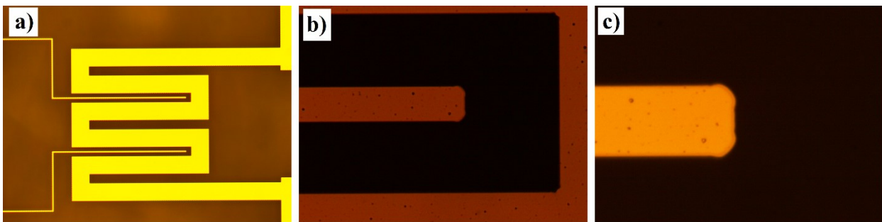
Figure 3.23: Metal interdigitate electrode over quartz wafers, process P1Q, with a magnification of a) 5x, b) 50x, and c) 100x.
