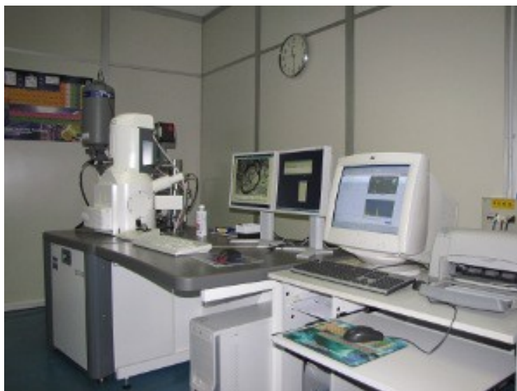
Figure 2.2: SEM Zeiss model EVO 40, available at the microscope centre of Ferrara [2.5].
