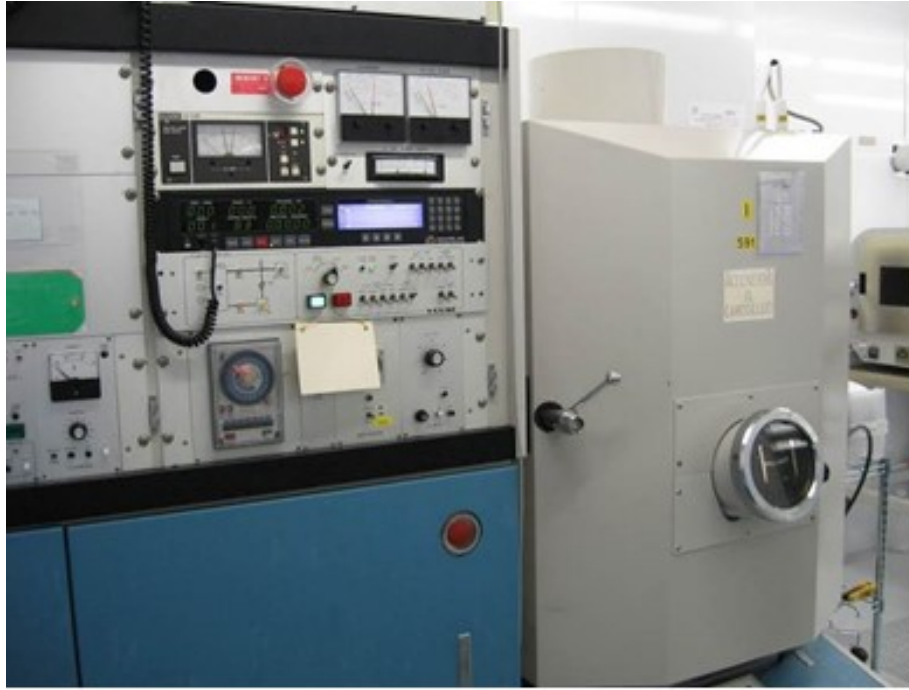
Figure 3.16: The PVD Ulvac, model EBX-16C, with e-gun Ferrotec EV S-6, available at the FBK.
