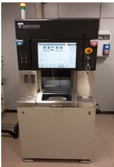
Figure 3.64: The Disco DAD 3650 Dicing Saw used in FBK for wafers dicing.
