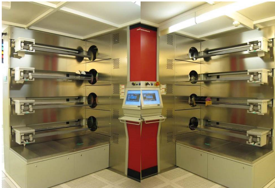
Figure 3.10: Horizontal tubes used in FBK for thermal oxidation and LPCVD processes.
