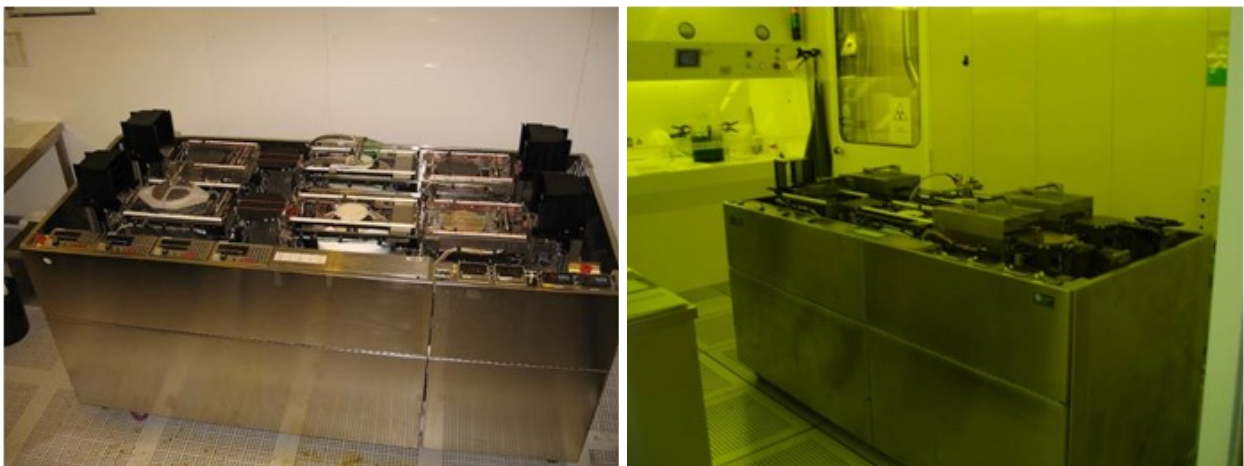
Figure 3.11: SVG 8600 Photoresist Coat Tracks available in FBK for photoresist coating and developing.
