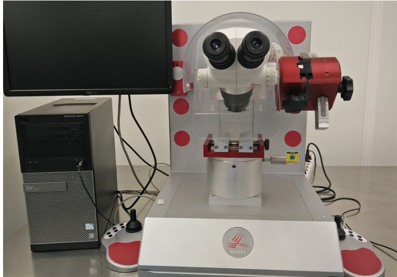
Figure 3.51: XYZTEST Condor Ez Bond Tester, present in the FBK, used for shear and pull tests.
