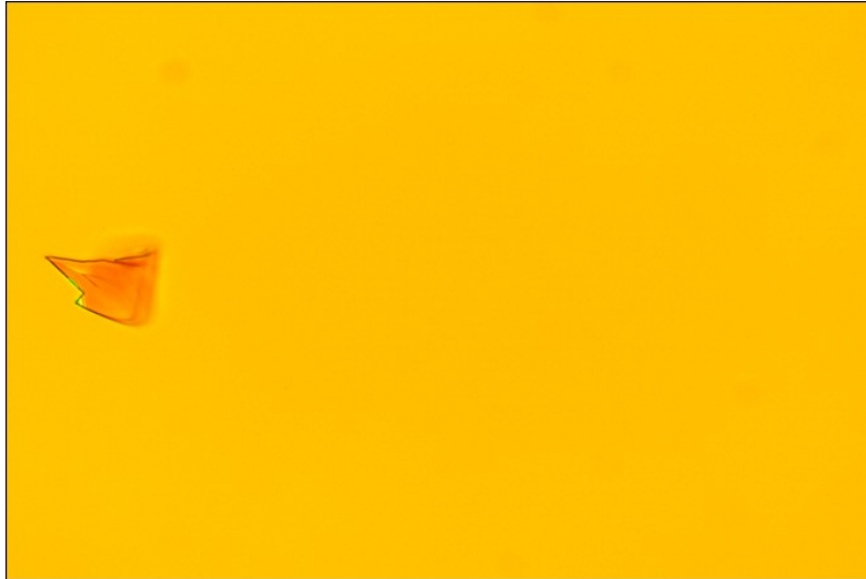
Figure 3.27: Image of surface peeling of 200 nm SiO 2 HF at 800°C (magnification 100x).
