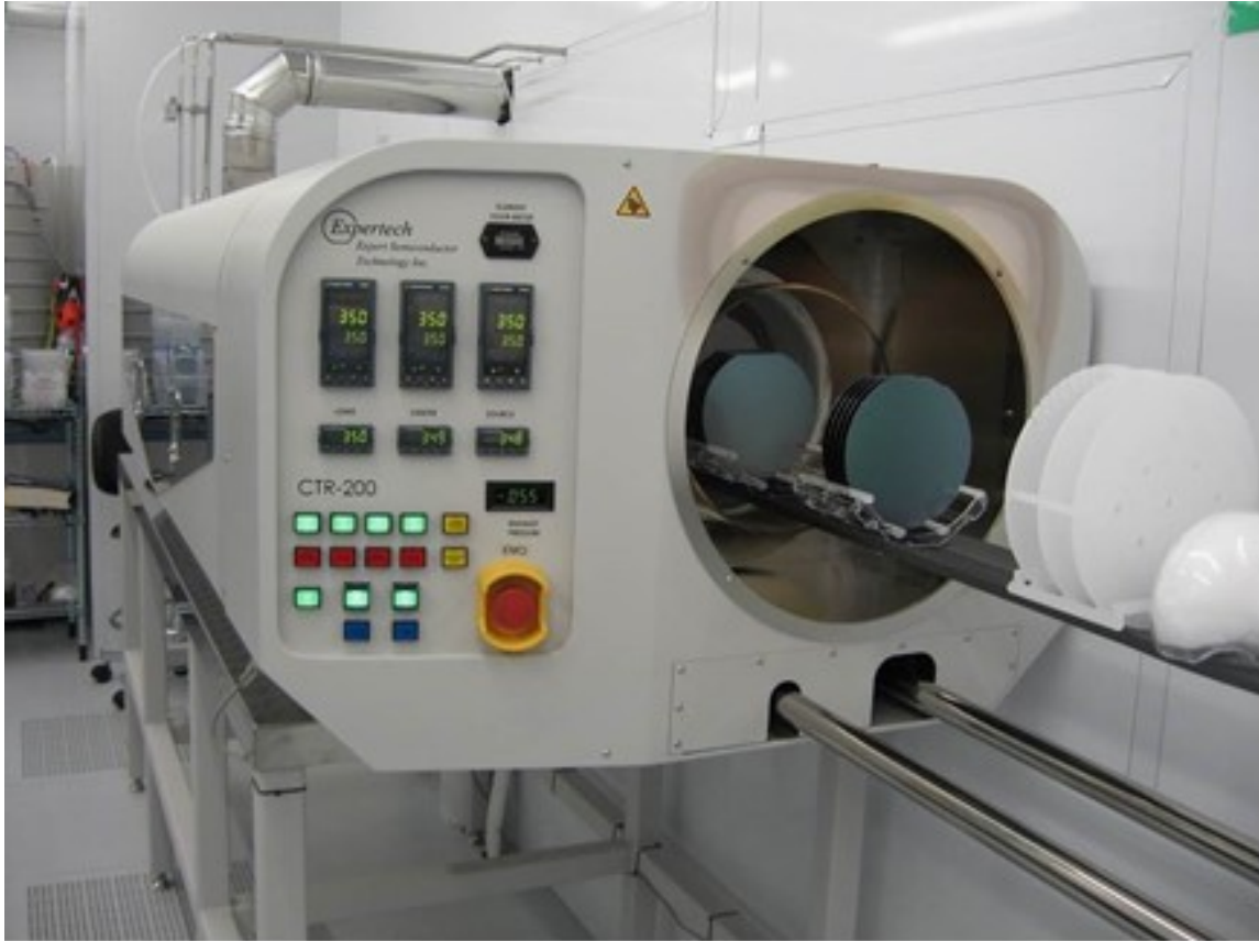
Figure 3.17: The Expertech Furnace for heat treatments at the FBK.
