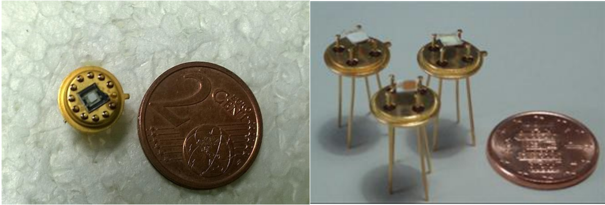
Figure 2.15: Bonded silicon substrate sensors, compared with a 2-cent money (left), and comparison between the bonded sensor and 1cent money (right).
