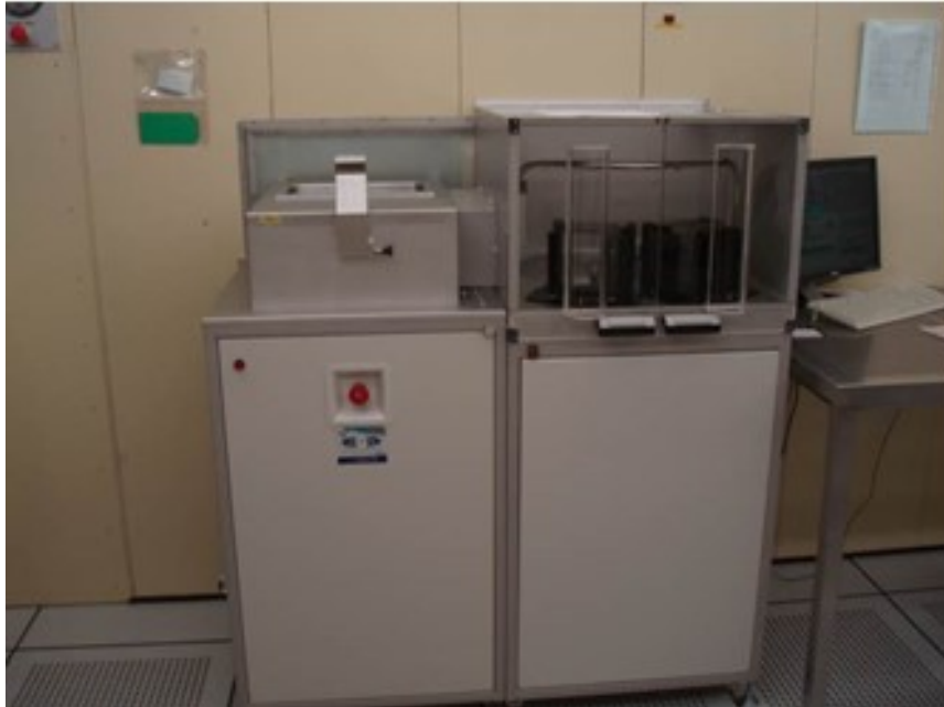
Figure 3.18: STS-MPS PECVD instrument available at the FBK.
