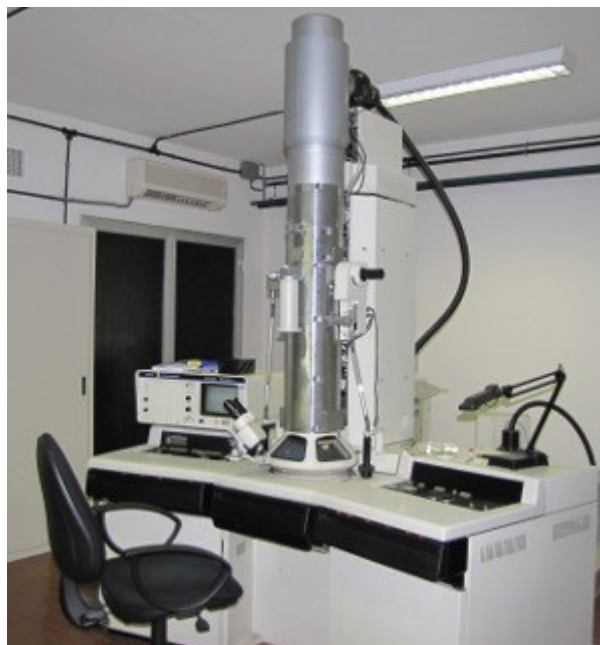
Figure 2.3: TEM Hitachi model H 800, available at the microscope centre of Ferrara.
