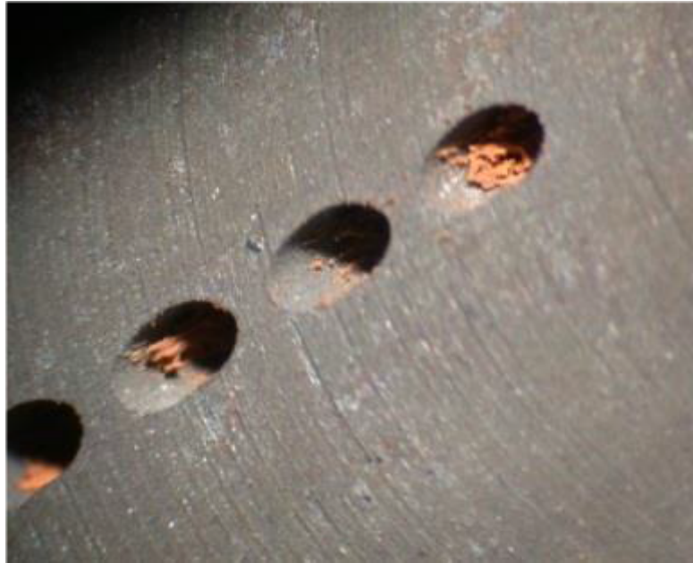
Figure 7.6: Internal cooling hole clogging Wylie et al. (2017): deposition in first four cooling holes of HD45 running at 1310 K
