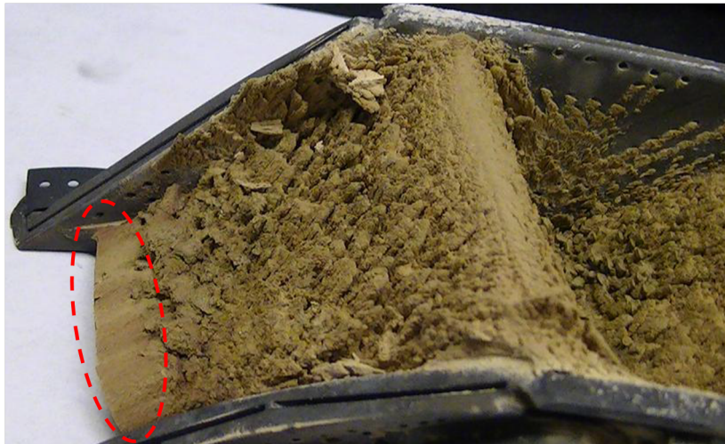
Figure 5.14: Fouled geometry from Webb et al. (2012): particular of the thin deposit in the trailing edge area
