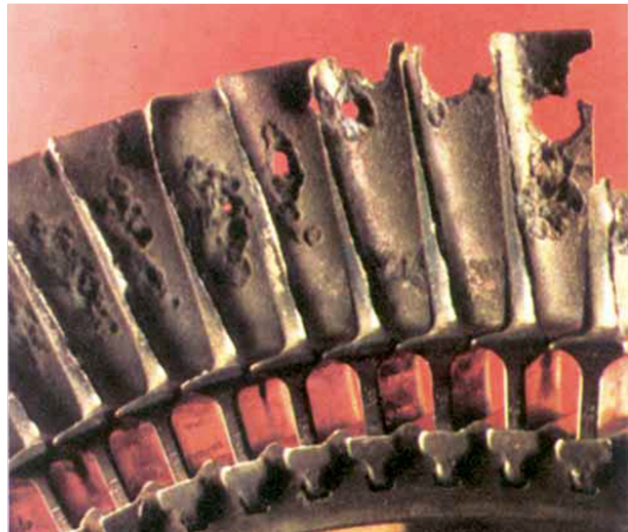
Figure 1.9: Cold-corrosion pitting on 403 Stainless Steel rotor blades (left, from Linden et al. 2001) And hot corrosion on turbine blades (right, from Wing and McGill 1981 )
