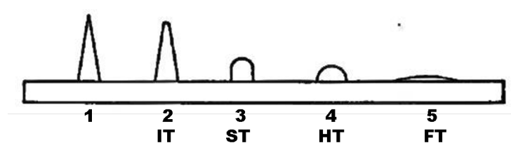
Figure 7.4: Critical temperature points. From Standard (2003)
