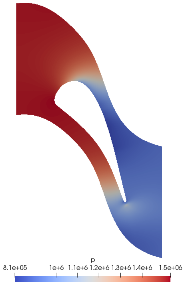
Figure 5.25: Pressure distribution on the fouled profile
