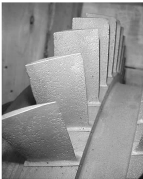
Figure 1.9: Cold-corrosion pitting on 403 Stainless Steel rotor blades (left, from Linden et al. 2001) And hot corrosion on turbine blades (right, from Wing and McGill 1981 )
