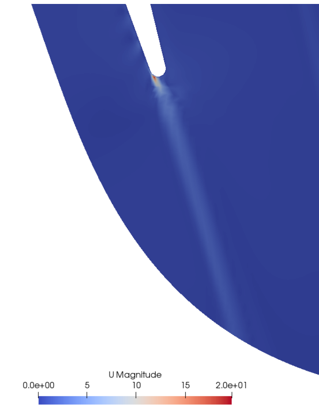
Figure 5.27: Wake variation due to deposition
