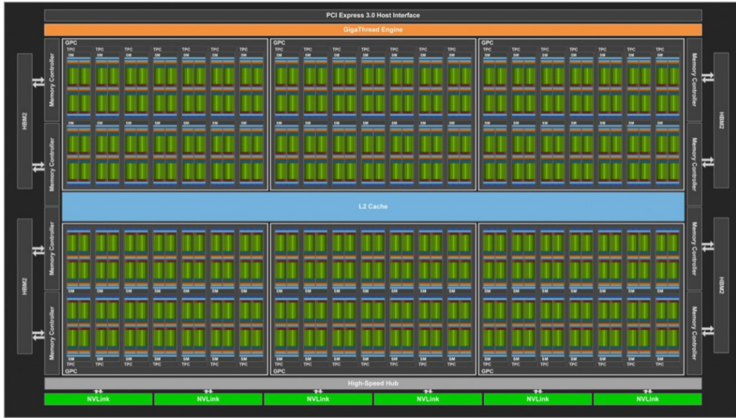
Figure 3.3: A modern GPU from Nvidia. It contains 5120 Cuda core FP32 and 2560 Cuda core FP64
