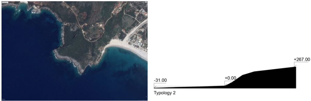
Figure 5.13 Coastal typology 2: Rock beach with high inclination, plan and section (source: author, based on Google Earth)
