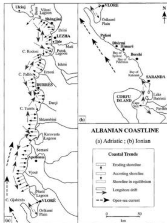
Figure 1 – Index map of the coast of Albania with indications of eroding and accreting sectors: (a) Adriatic Coast, (b) Ionian Coast.
